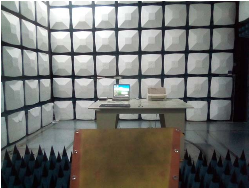
Radiated Emissions Above 1G front View
