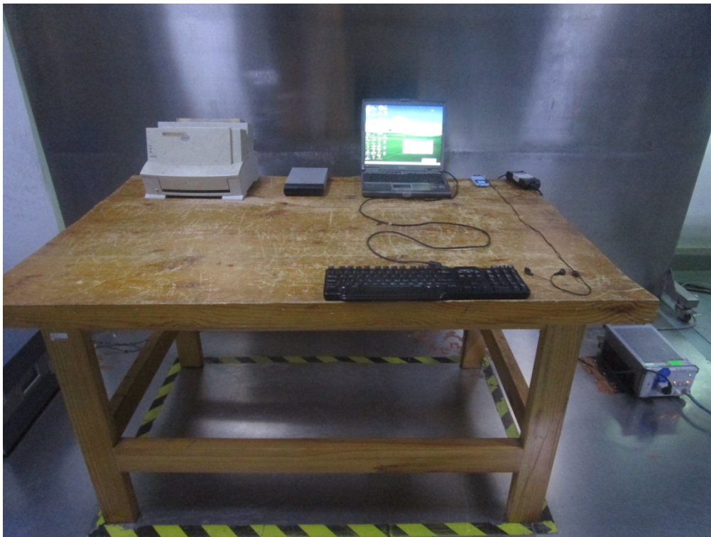
Conducted Emissions Front View
