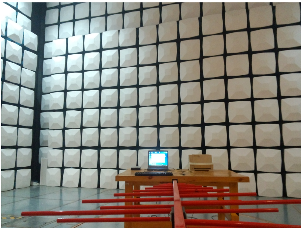
Radiated Emissions Below 1G front View
