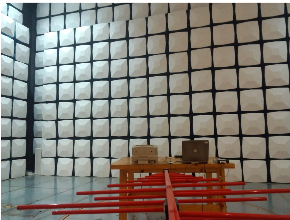
Radiated Emissions Below 1G Rear View
