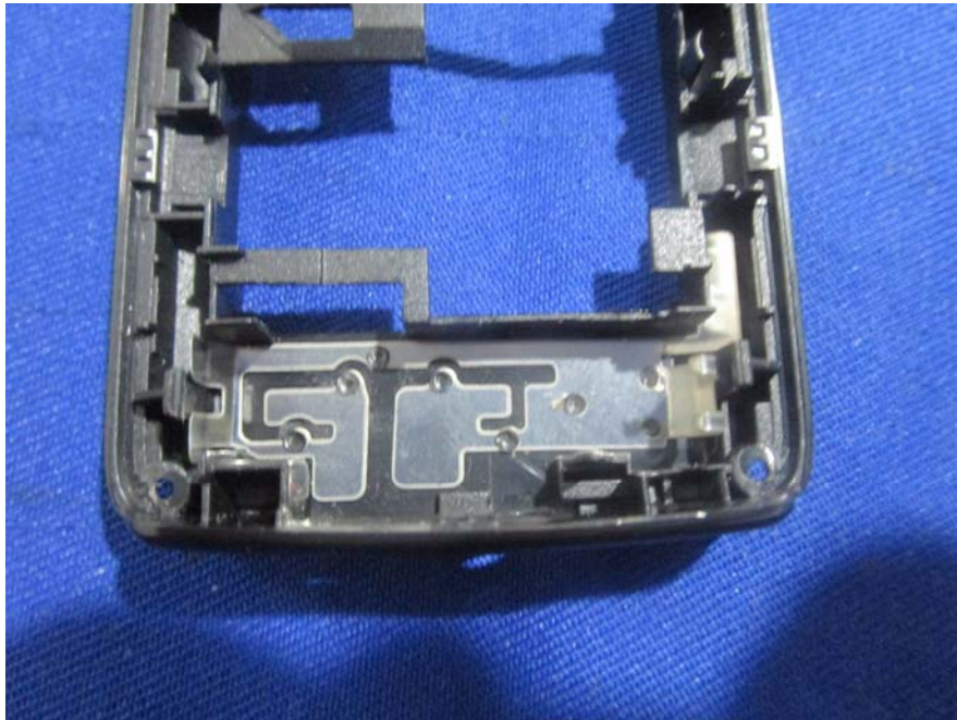
EUT – GPS Antenna View
