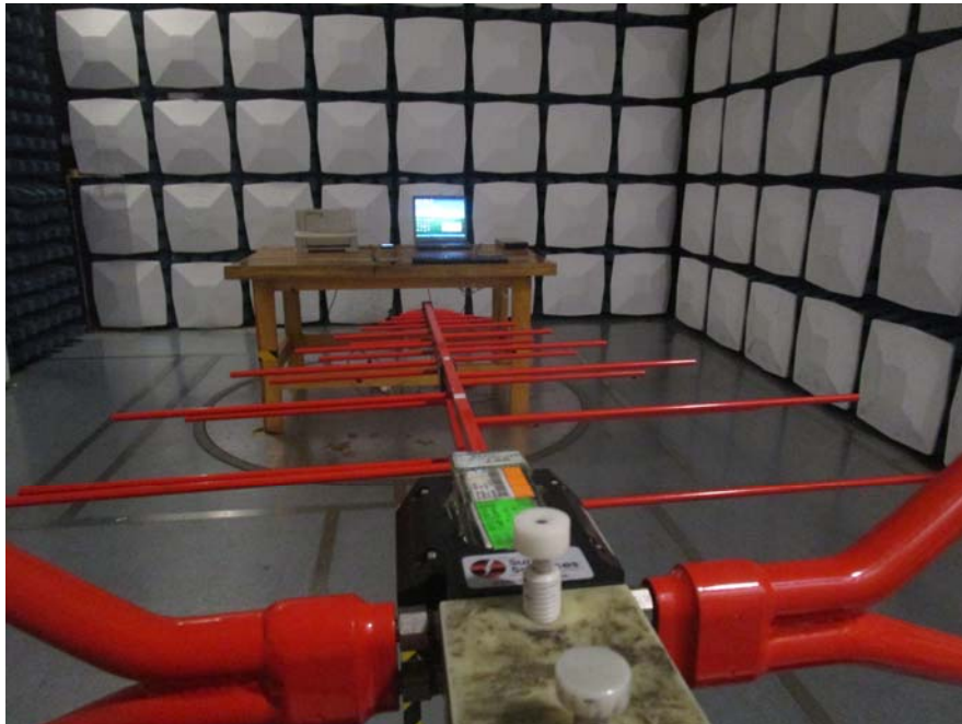
Radiated Emission Below 1GHz – Front View
