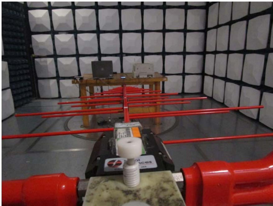
Radiated Emission Below 1GHz – Rear View
