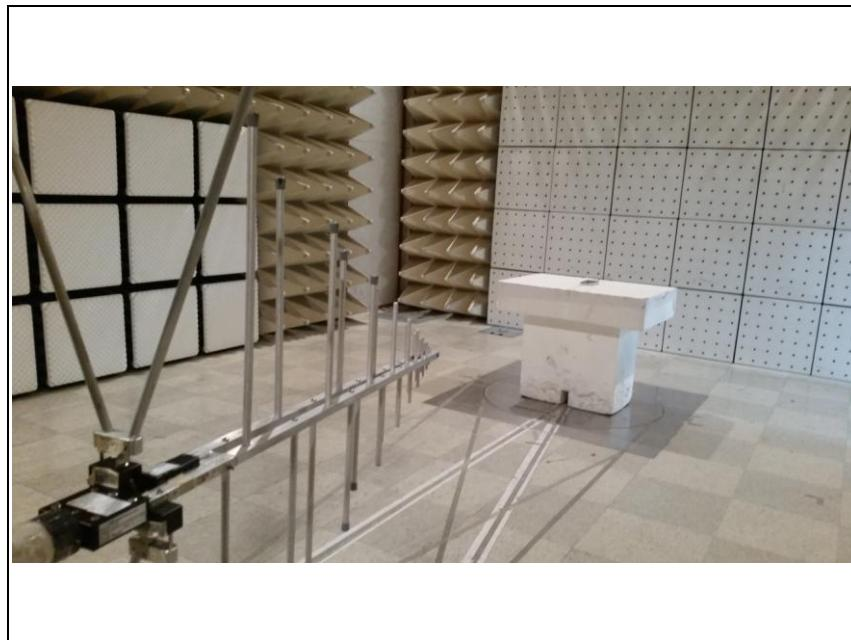
**C. The photos of E-field test with Resistive load.**
