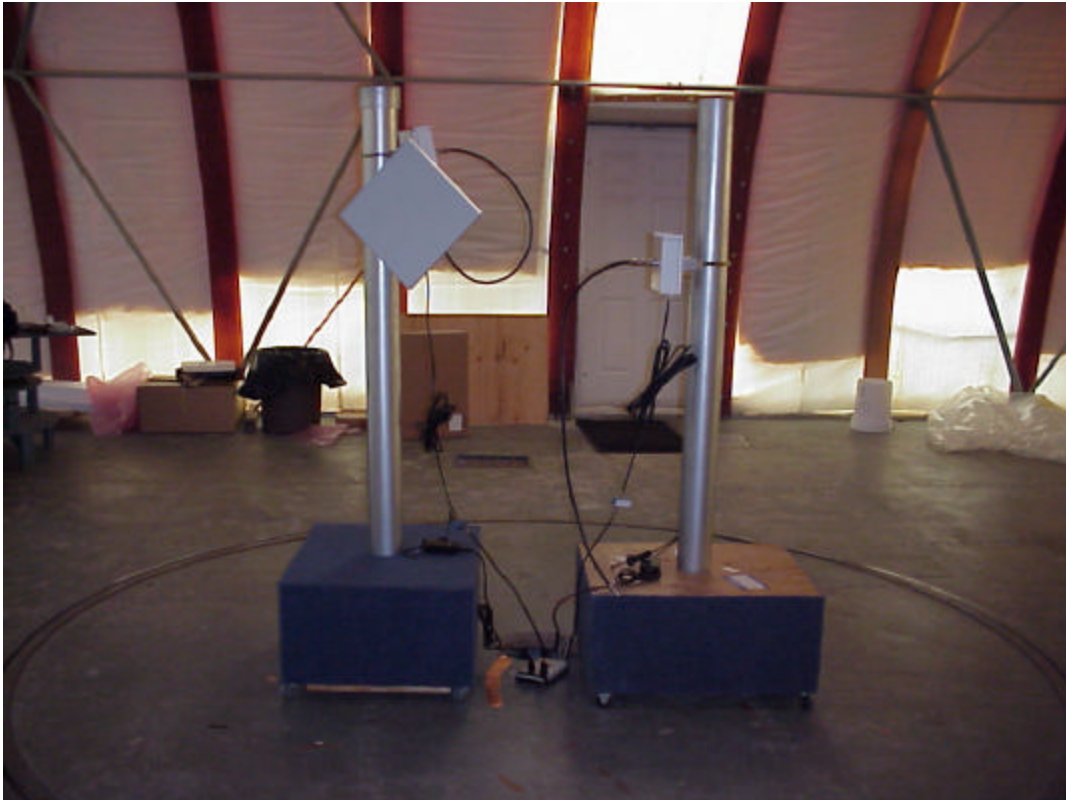
Flat Panel Point-to-Point 23 dBi Gain
