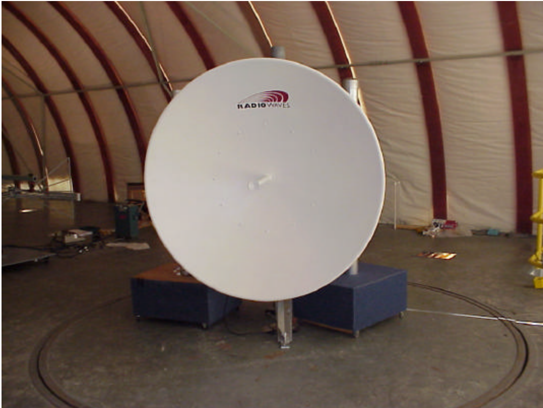
6' Parabolic Point-to-Point 37.6 dBi Gain
