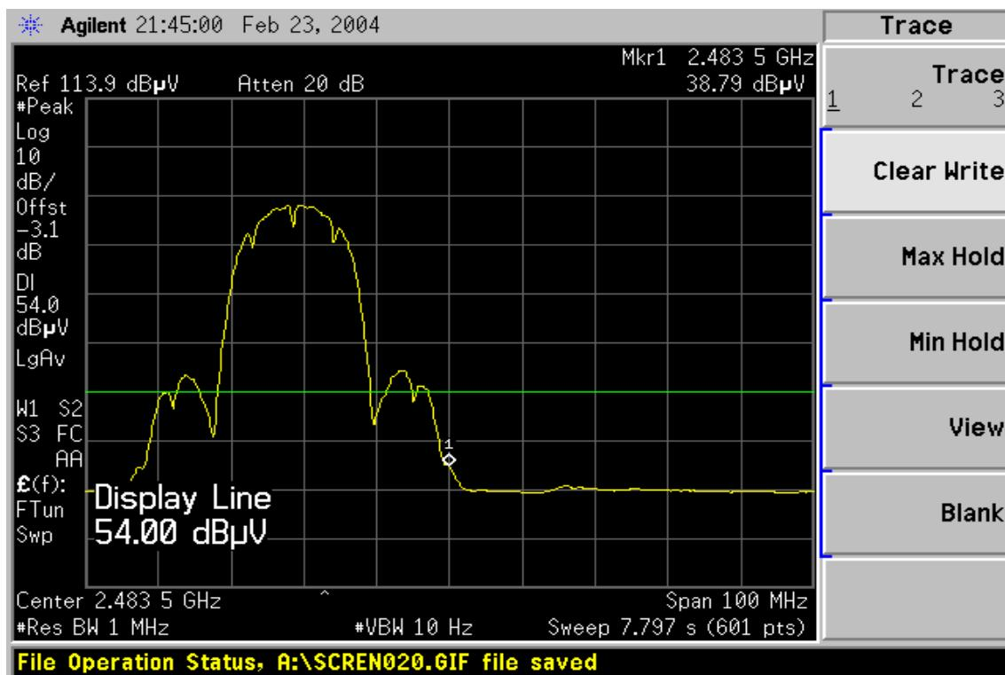
**Band Edges (IEEE 802.11g / CH Low)****Detector mode: Peak****Polarity: Vertical**
