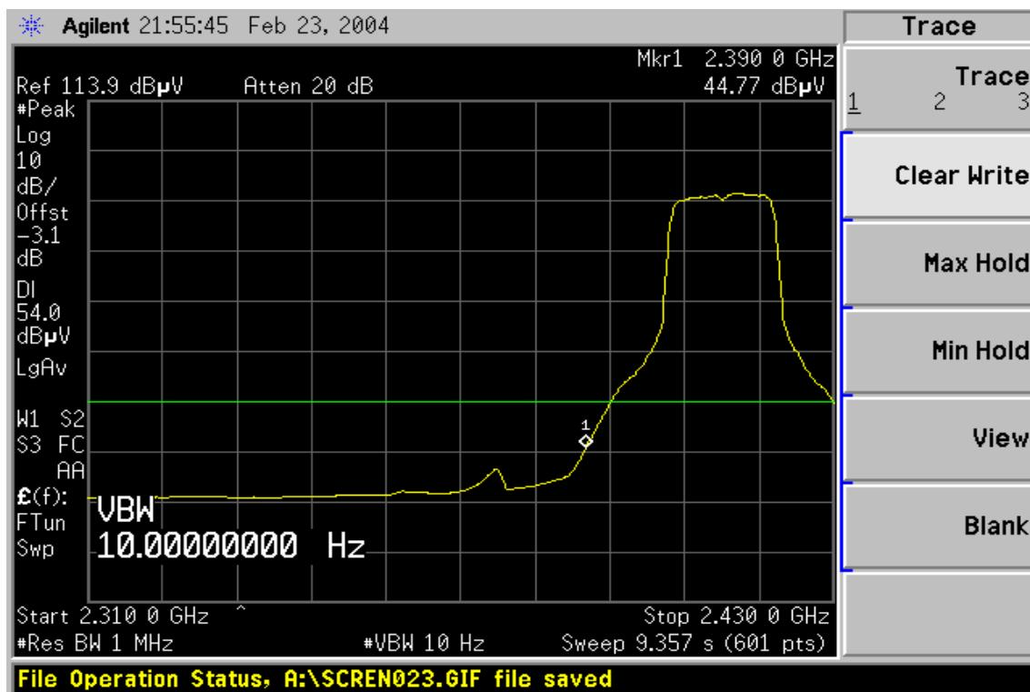
**Band Edges (IEEE 802.11g / CH High)****Detector mode: Peak****Polarity: Vertical**
