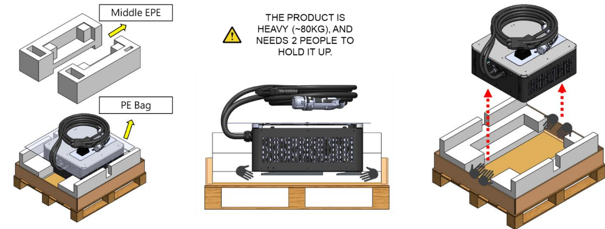
Figure 1-7 Take Out the Middle EPE and Lift the Wallbox
