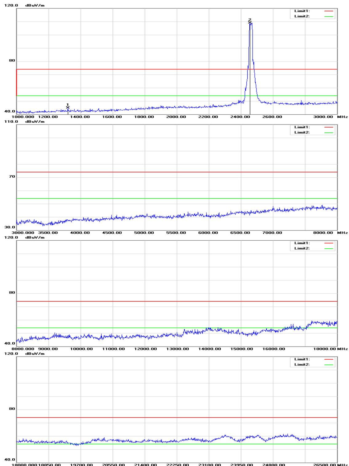
**Operation Mode:** TX / IEEE 802.11g / 2462 MHz**Test Date:** January 11, 2016**Temperature:** 27°C**Tested by:** Jason Lu**Humidity:** 53% RH**Polarity:** Ver. / Hor.
