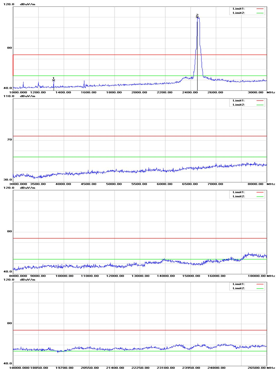
**Operation Mode:** TX / IEEE 802.11n HT 20 MHz mode / 2462 MHz
