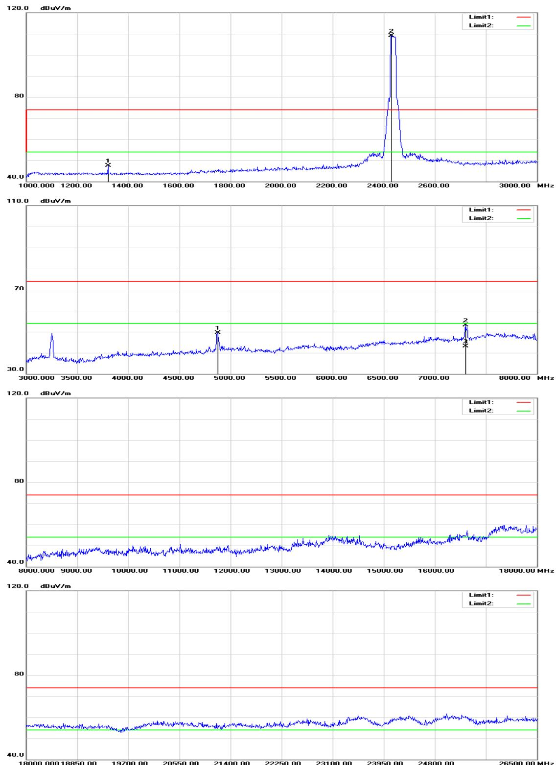
**Operation Mode:** TX / IEEE 802.11n HT 20 MHz mode / 2437 MHz
