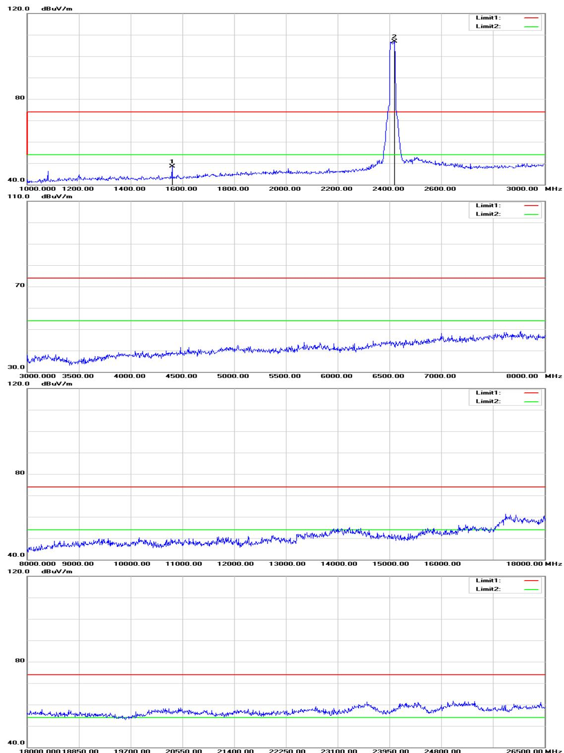
**Operation Mode:** TX / IEEE 802.11n HT 20 MHz mode / 2412 MHz
