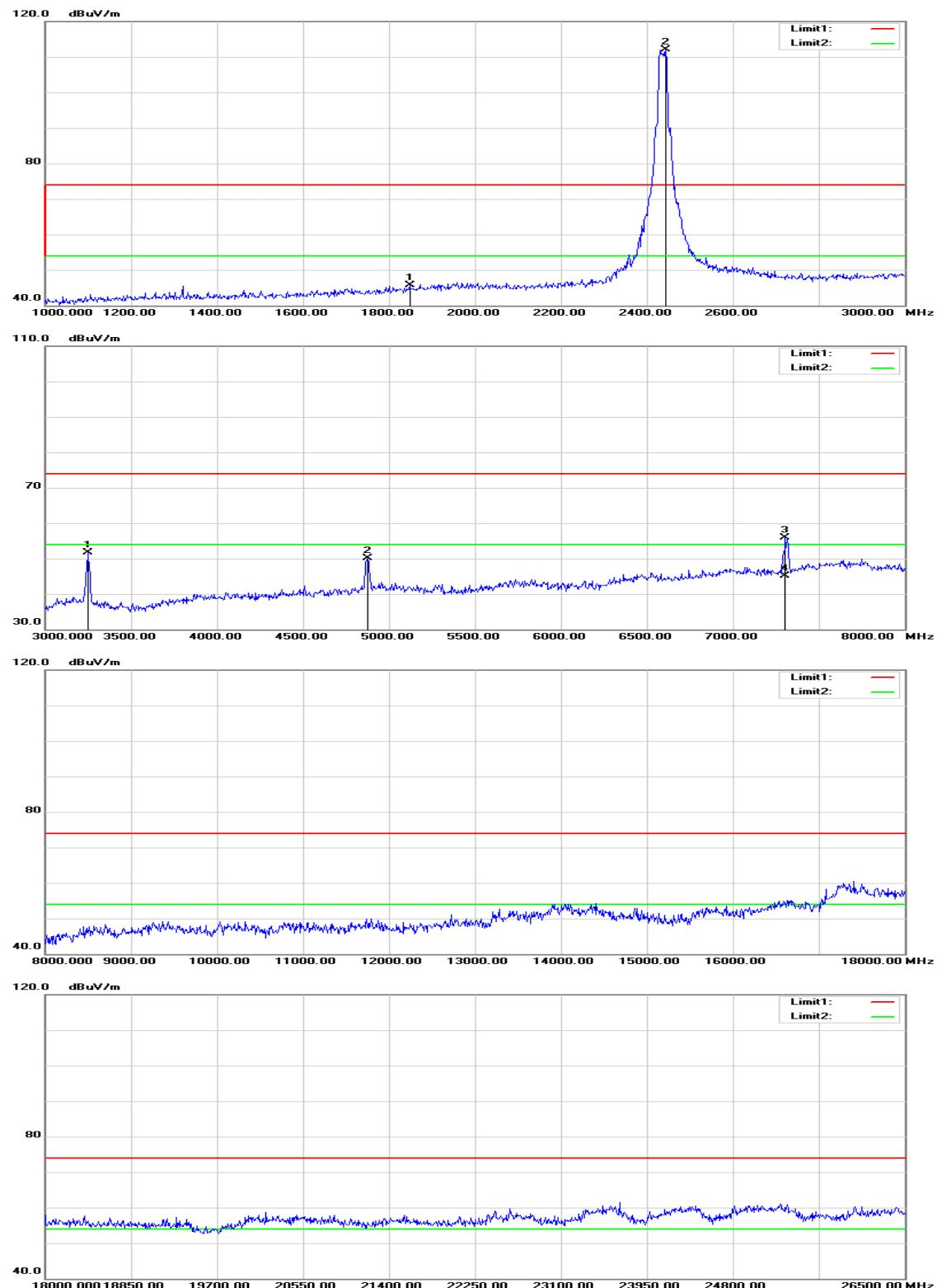
**Operation Mode:** TX / IEEE 802.11g / 2437 MHz**Test Date:** January 11, 2016**Temperature:** 27°C**Tested by:** Jason Lu**Humidity:** 53% RH**Polarity:** Ver. / Hor.
