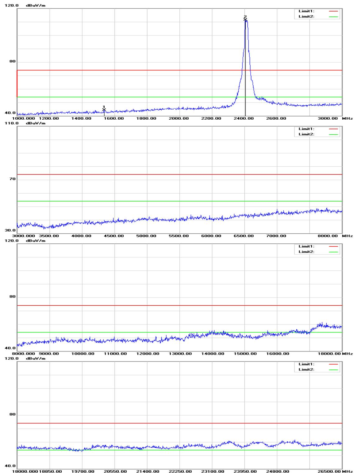
**Operation Mode:** TX / IEEE 802.11g / 2412 MHz**Test Date:** January 11, 2016**Temperature:** 27°C**Tested by:** Jason Lu**Humidity:** 53% RH**Polarity:** Ver. / Hor.
