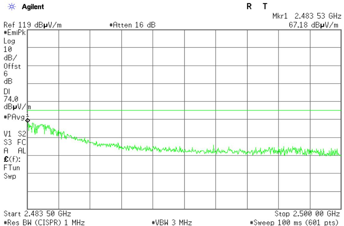
**Detector mode: Average****Polarity: Vertical**
