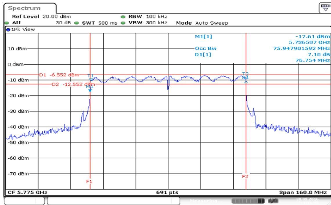
**IEEE 802.11ac VHT 80 MHz mode / 5775MHz / Chain 1****99% Bandwidth (CH Mid)**
