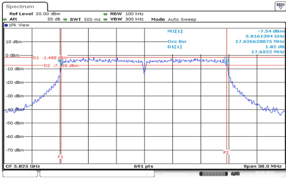
**IEEE 802.11n HT 40 MHz mode / 5755 ~ 5795MHz / Chain 0****99% Bandwidth (CH Low)**
