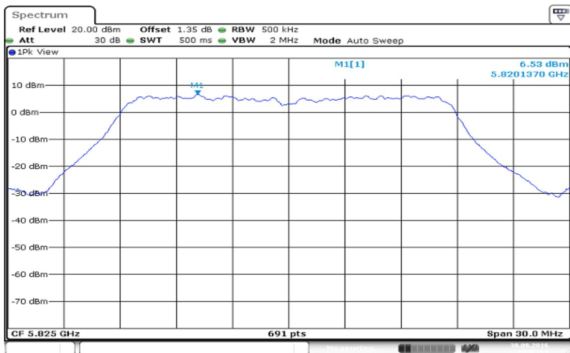
**IEEE 802.11n HT 20 MHz mode / 5745 ~ 5825MHz / Chain 1****PPSD (CH Low)**
