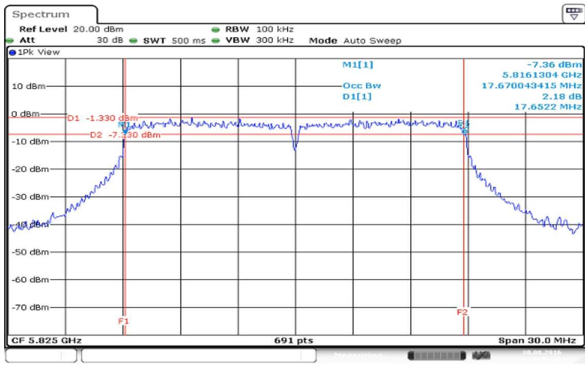
**IEEE 802.11n HT 20 MHz mode / 5745 ~ 5825MHz / Chain 1****6dB Bandwidth (CH Low)**
