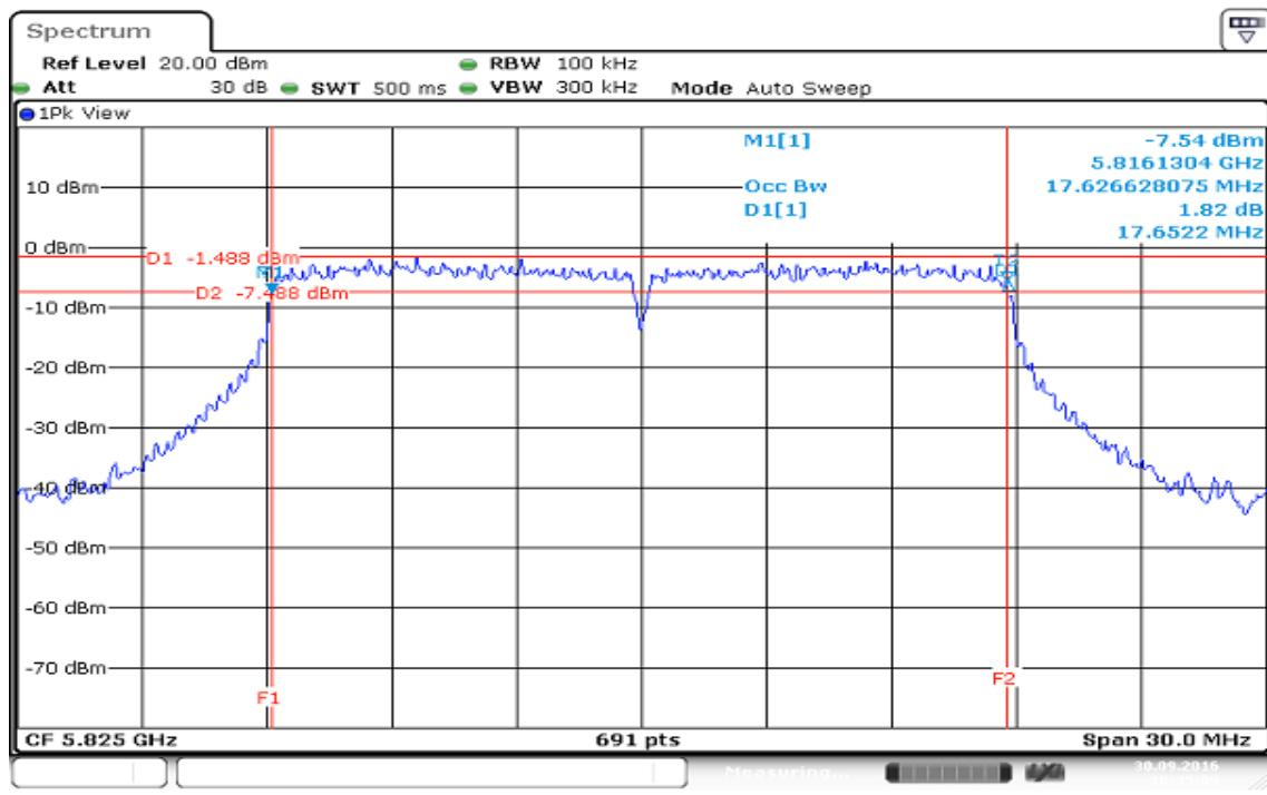
**IEEE 802.11n HT 40 MHz mode / 5755 ~ 5795MHz / Chain 0****6dB Bandwidth (CH Low)**
