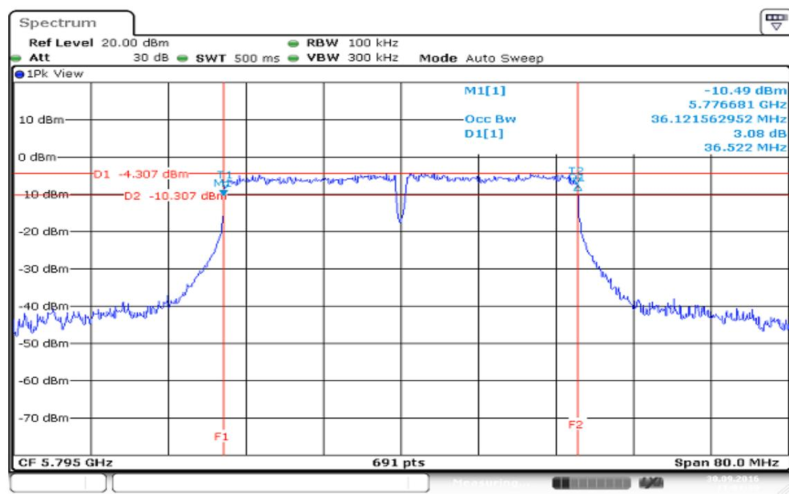
**IEEE 802.11n HT 40 MHz mode / 5755 ~ 5795MHz / Chain 1****99% Bandwidth (CH Low)**
