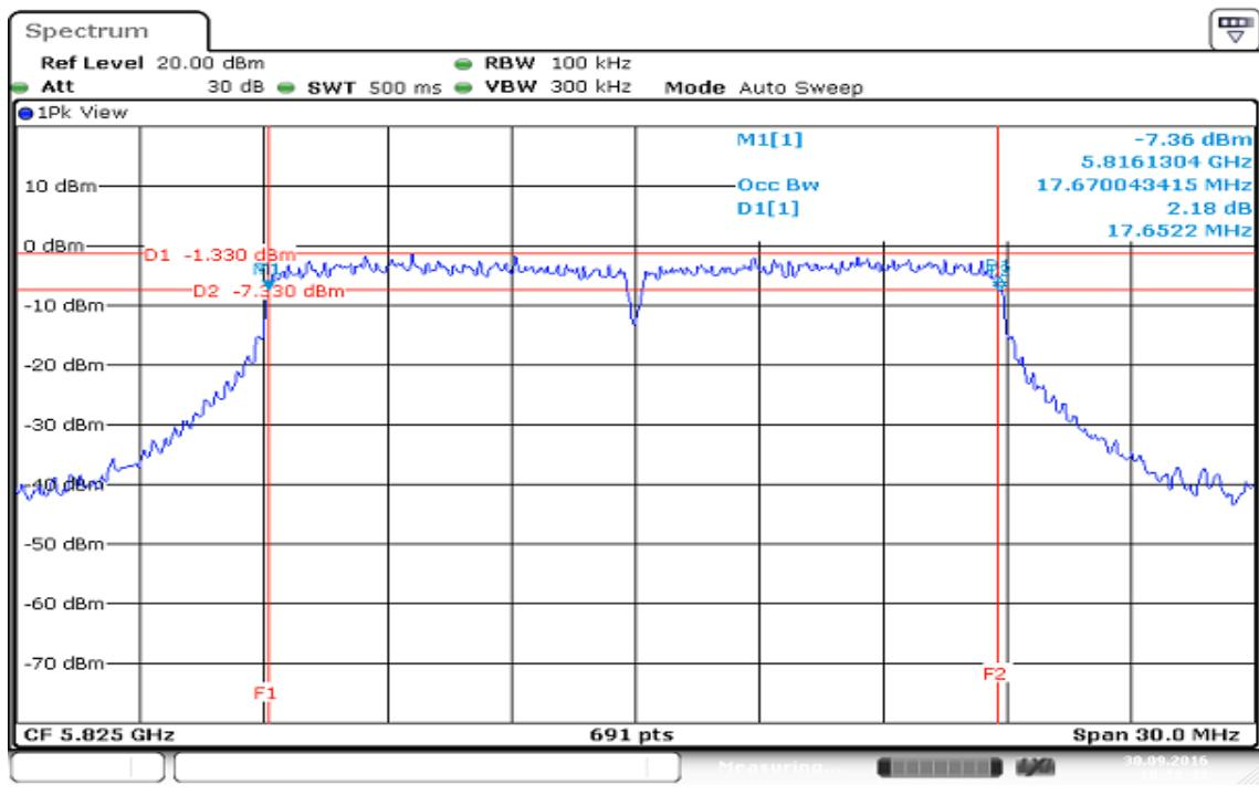
**IEEE 802.11n HT 20 MHz mode / 5745 ~ 5825MHz / Chain 1****99% Bandwidth (CH Low)**
