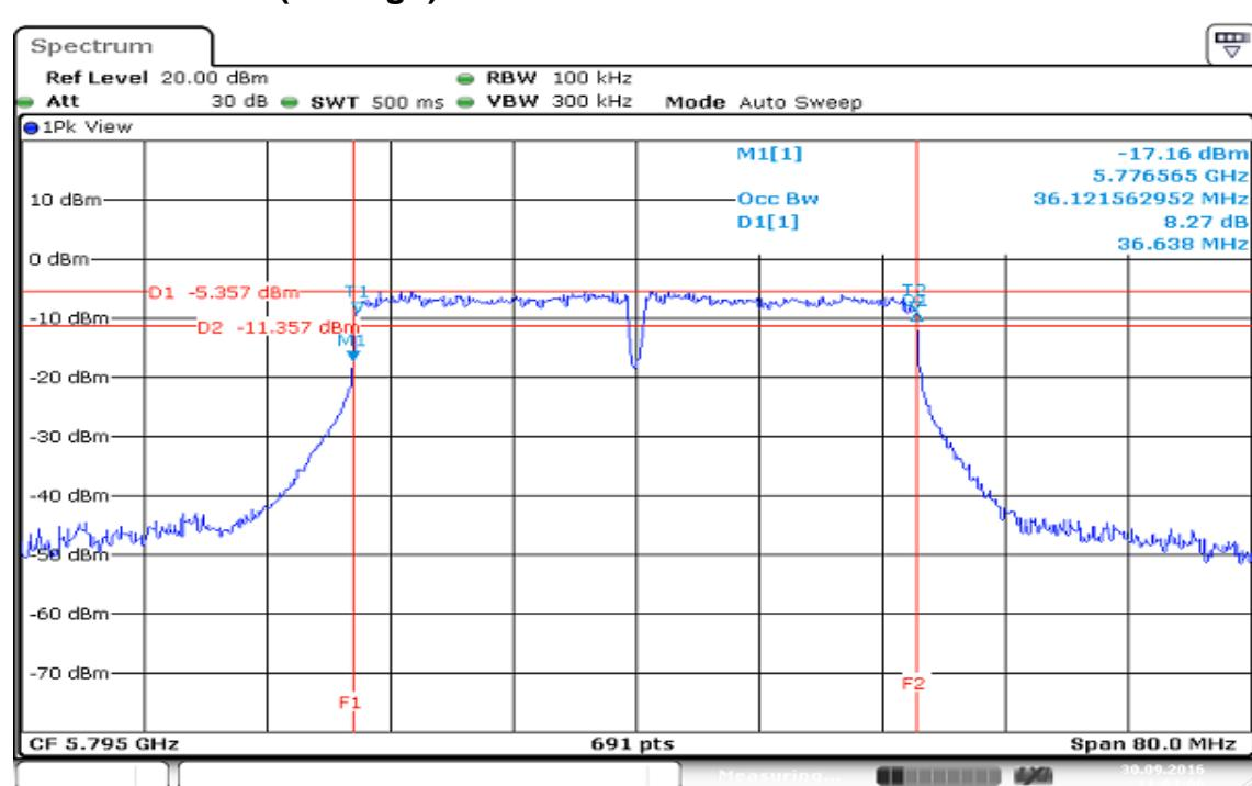
**IEEE 802.11ac VHT 80 MHz mode / 5775MHz / Chain 0****6dB Bandwidth (CH Mid)**
