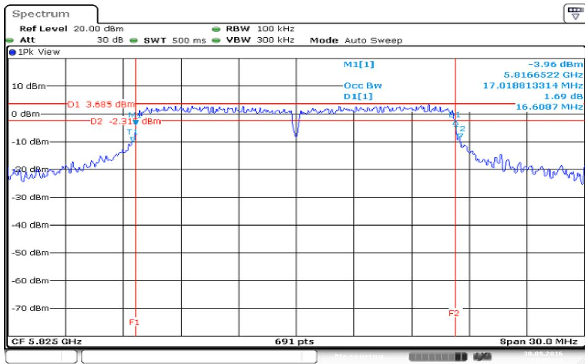
**IEEE 802.11n HT 20 MHz mode / 5745 ~ 5825MHz / Chain 0****6dB Bandwidth (CH Low)**
