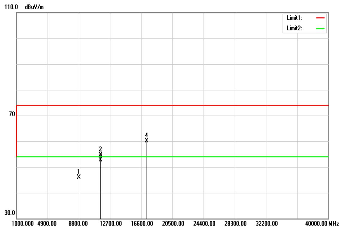
**Operation Mode:** Tx / IEEE 802.11ac VHT 80 MHz mode / CH Mid **Test Date:** September 30, 2016
