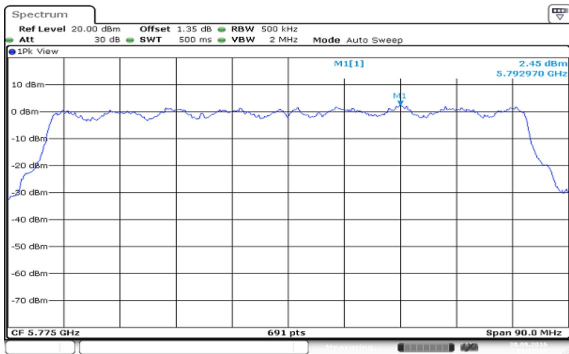
**IEEE 802.11ac VHT 80 MHz mode / 5775MHz / Chain 1****PPSD (CH Mid)**
