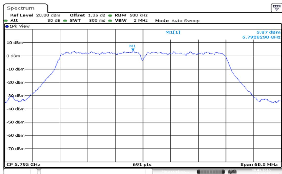
**IEEE 802.11ac VHT 80 MHz mode / 5775MHz / Chain 0****PPSD (CH Mid)**
