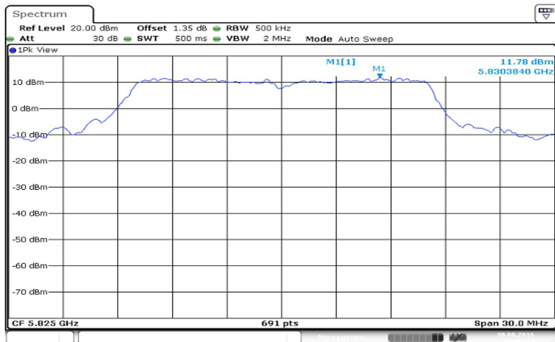
**IEEE 802.11n HT 20 MHz mode / 5745 ~ 5825MHz / Chain 0****PPSD (CH Low)**
