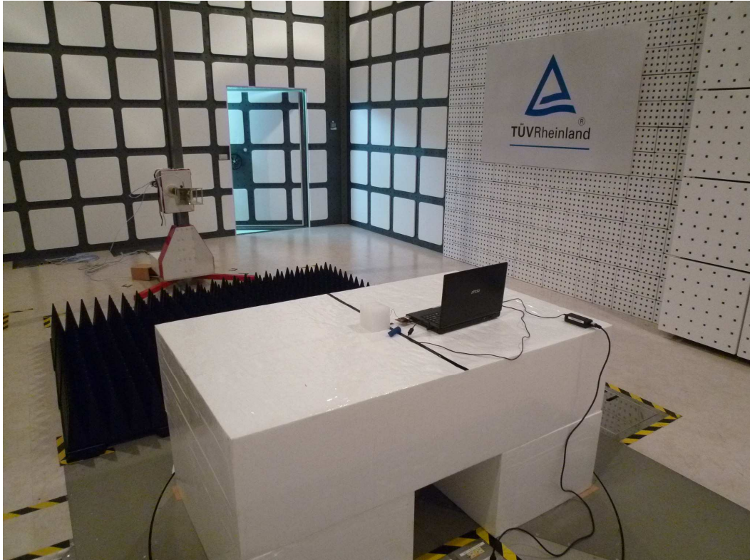
Photograph 4: Set-up for Conducted testing
