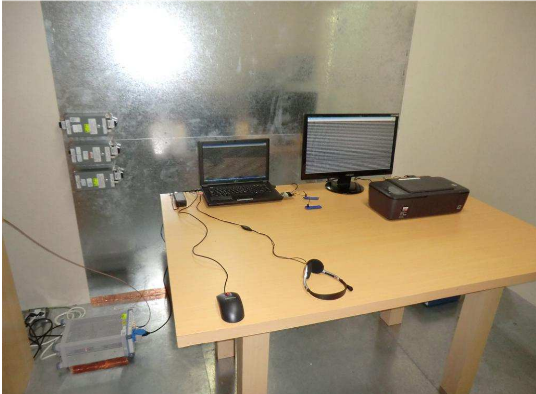
Photograph 6: Set-up for Mains Conducted Emissions (Back View)
