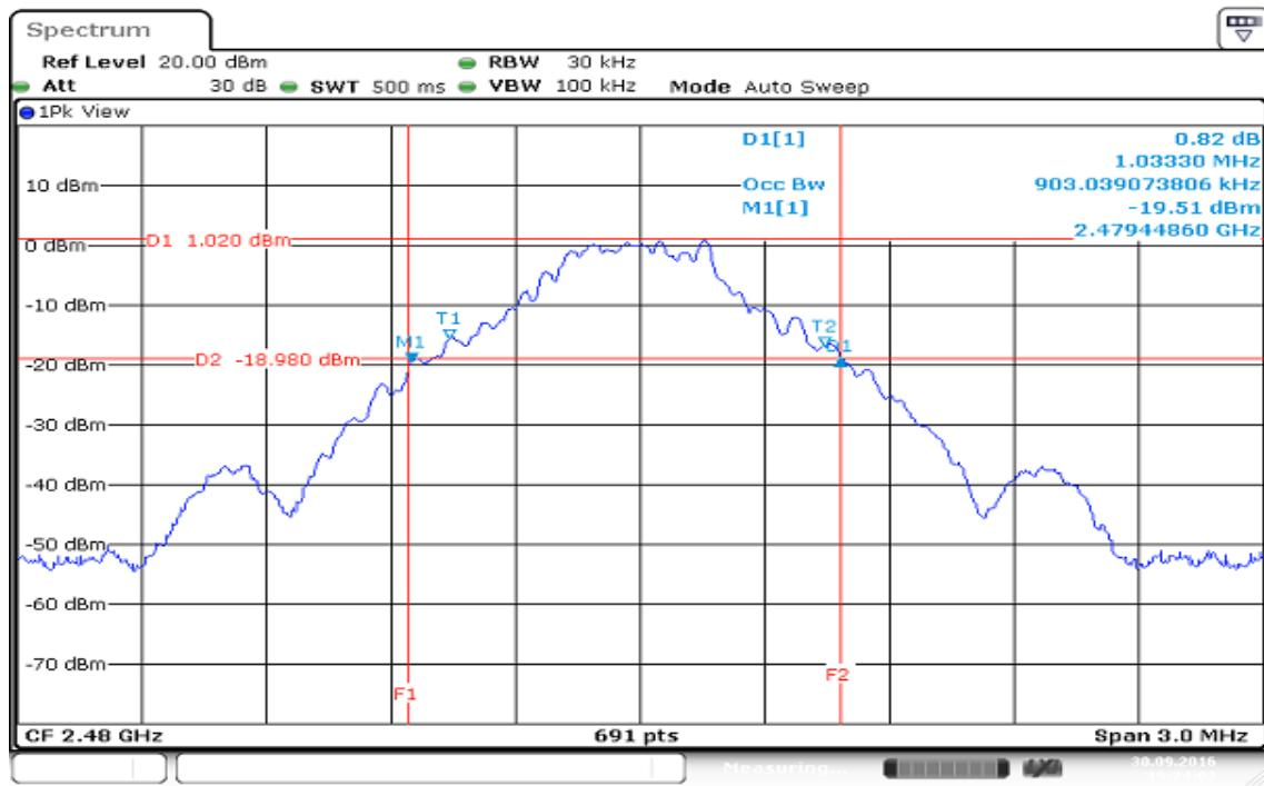
**For 8DPSK / DH5****99% Bandwidth (CH Low)**
