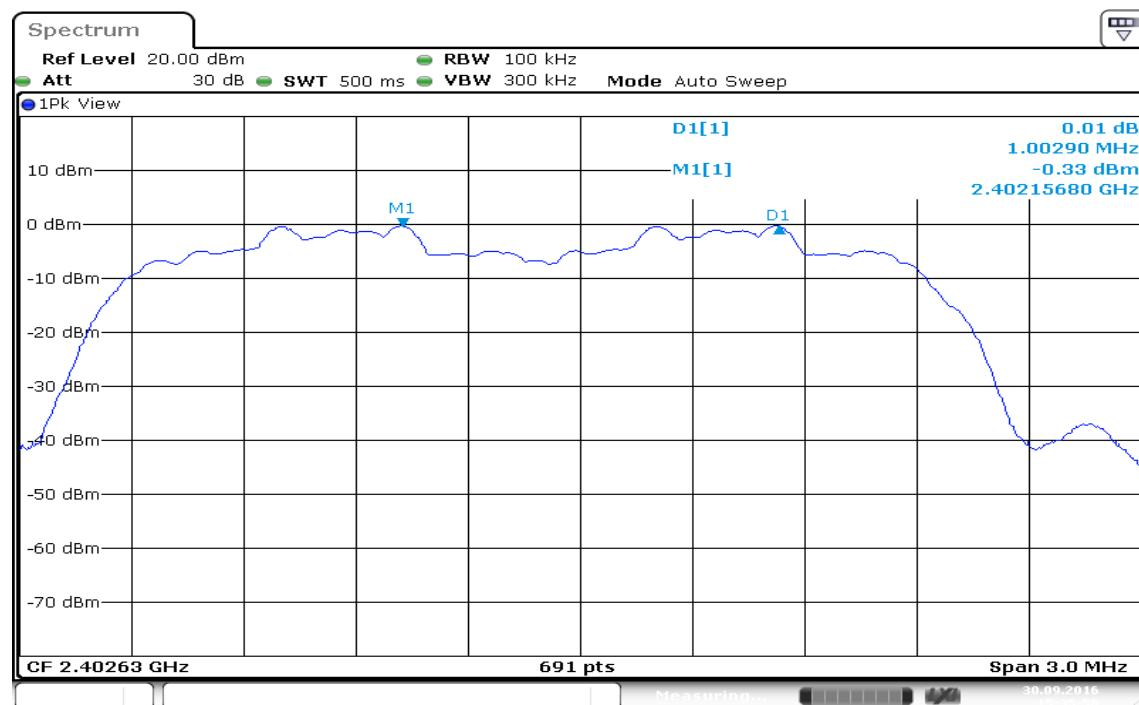
**Measurement of Channel Separation / (CH Mid)**
