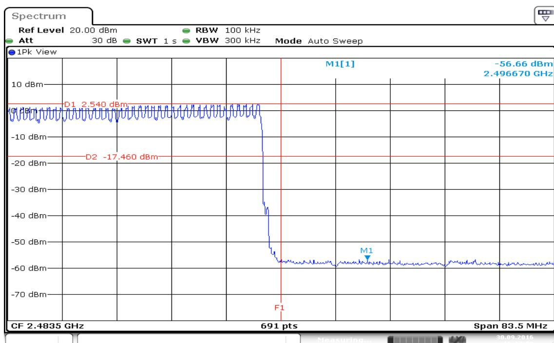
**Test Plot****For GFSK****Un-restricted Band Emissions / CH Low**
