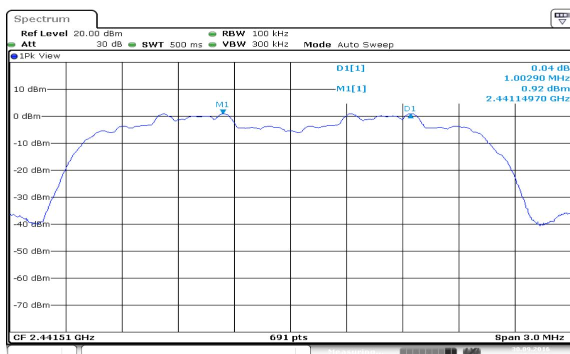
**Measurement of Channel Separation / (CH High)**
