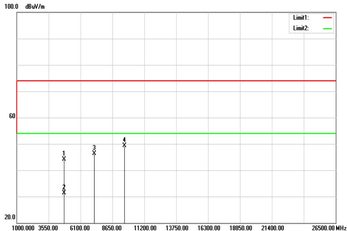
**Above 1 GHz****Operation Mode:** TX / DH5 / CH Low**Test Date:** September 22, 2016**Temperature:** 27°C**Tested by:** Dennis Li**Humidity:** 53 % RH**Polarity:** Ver. / Hor.
