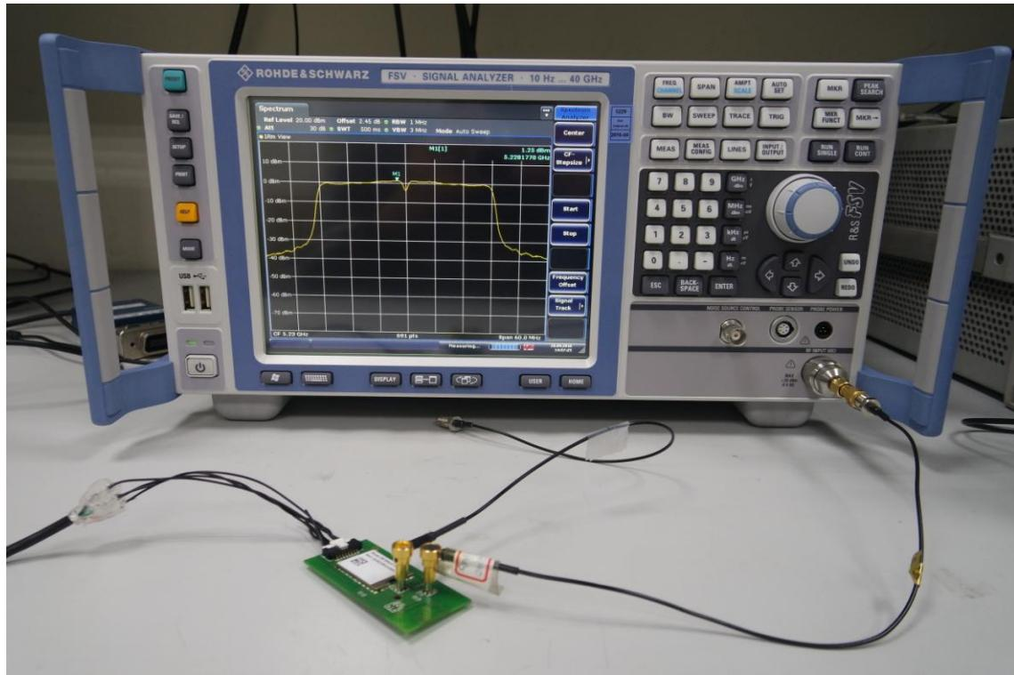
**RADIATED EMISSION SETUP PHOTOS****For PIFA Antenna****Below 1GHz**
