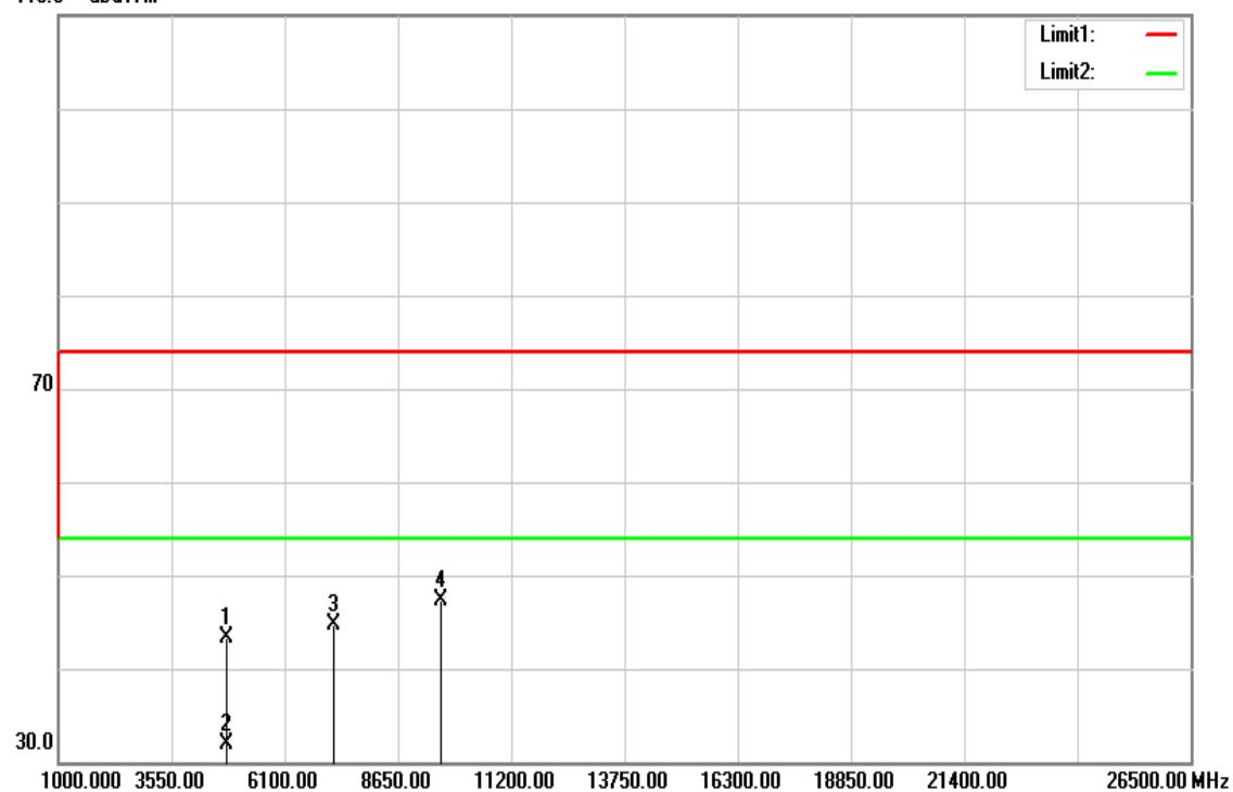
**Operation Mode:** GFSK / TX / CH Low**Test Date:** September 7, 2016**Temperature:** 27°C**Tested by:** Dennis Li**Humidity:** 53 % RH**Polarity:** Ver. / Hor.
