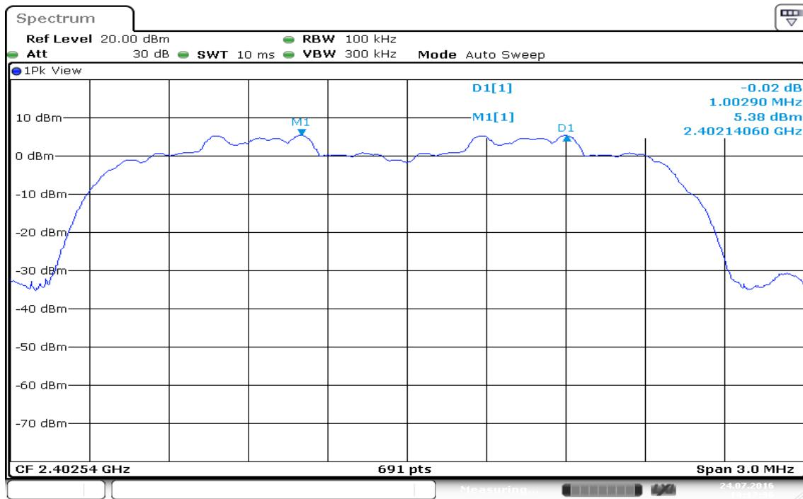
**Measurement of Channel Separation / (CH Mid)**
