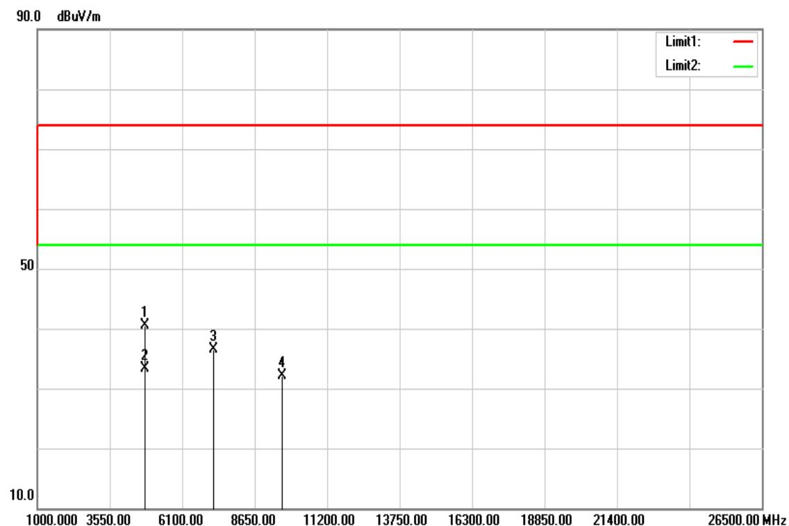
**Above 1 GHz****Operation Mode:** TX / DH5 / CH Low**Test Date:** July 29, 2016**Temperature:** 27°C**Tested by:** Dennis Li**Humidity:** 53 % RH**Polarity:** Ver. / Hor.
