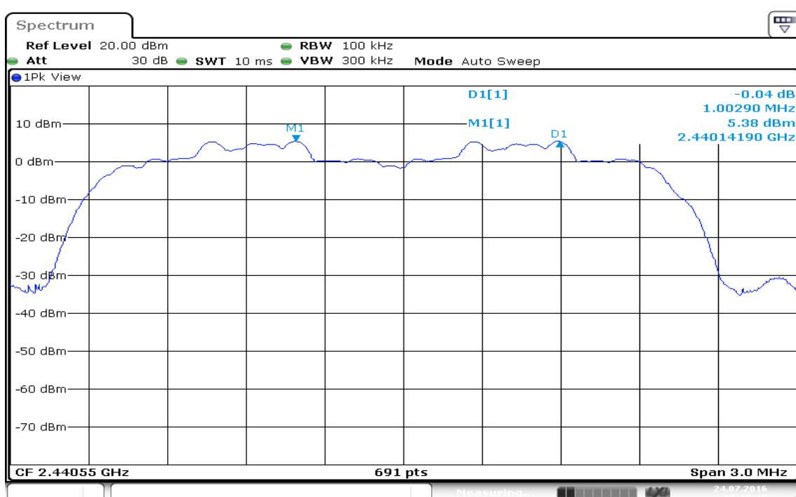
**Measurement of Channel Separation / (CH High)**
