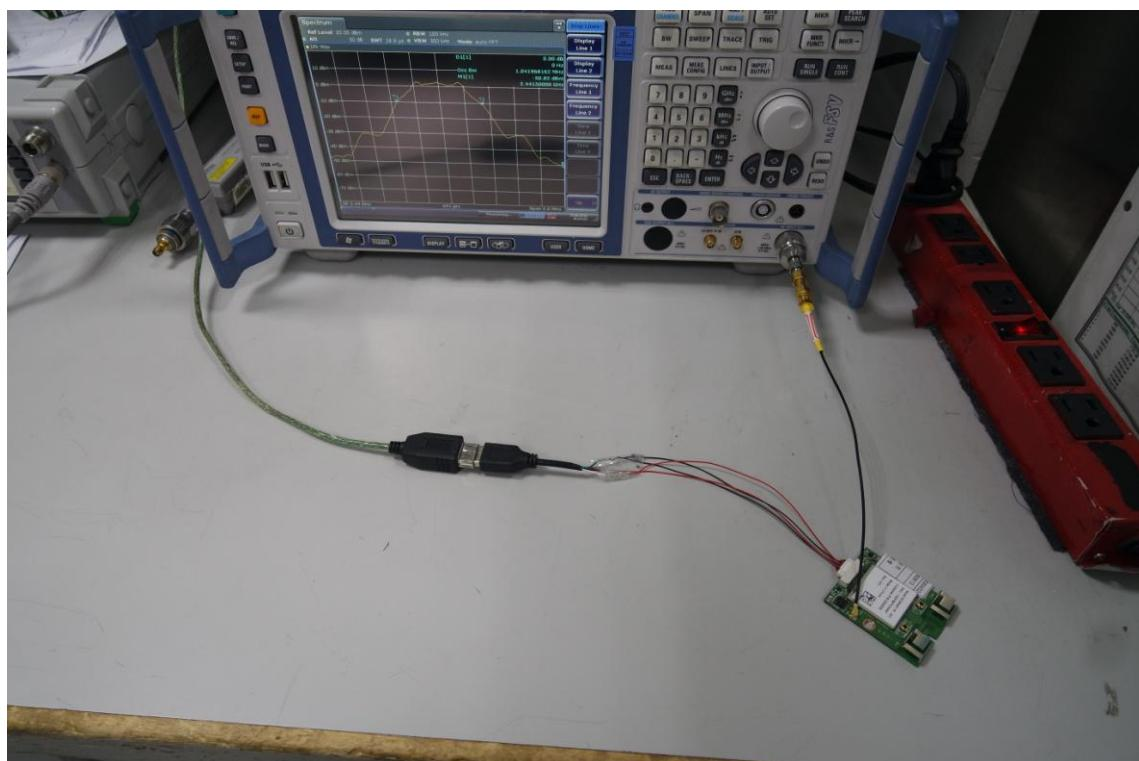
**Radiated Emissions Setup Photos****Below 1 GHz**
