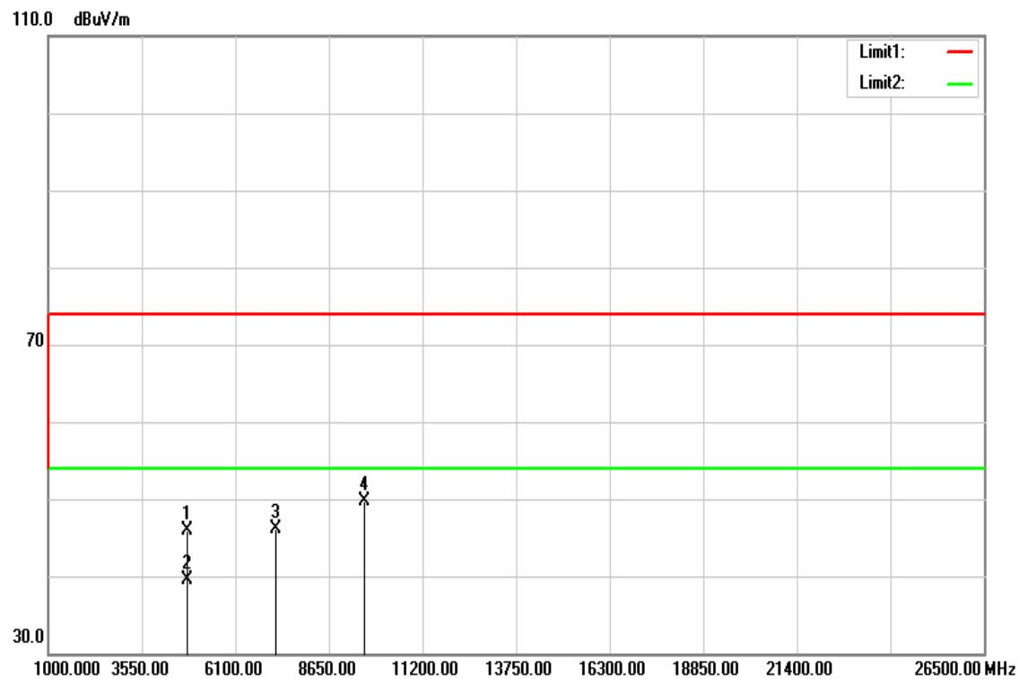
**Above 1 GHz****Operation Mode:** TX / DH5 / CH Low**Test Date:** November 15, 2016**Temperature:** 27°C**Tested by:** Dennis Li**Humidity:** 53 % RH**Polarity:** Ver. / Hor.
