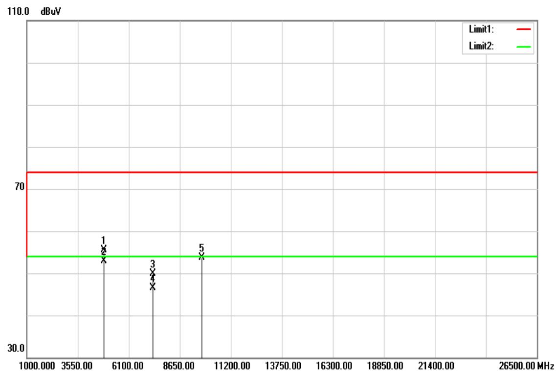
**Operation Mode:** TX / IEEE 802.11b / CH Mid**Test Date:** June 22, 2016**Temperature:** 27°C**Tested by:** Dennis Li**Humidity:** 53% RH**Polarity:** Ver. / Hor.
