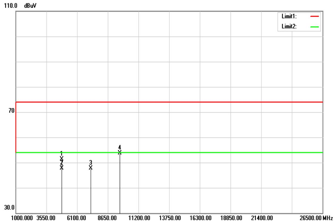
**Above 1 GHz****Operation Mode:** TX / IEEE 802.11b / CH Low**Test Date:** June 22, 2016**Temperature:** 27°C**Tested by:** Dennis Li**Humidity:** 53% RH**Polarity:** Ver. / Hor.
