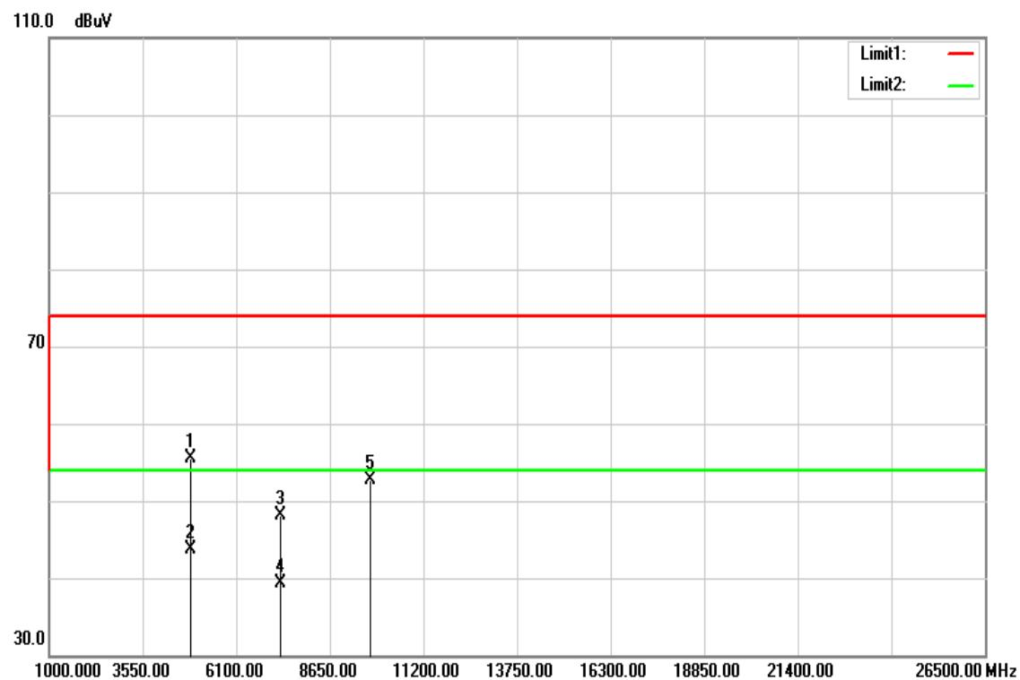
**Operation Mode:** TX / IEEE 802.11g / CH Mid**Test Date:** June 22, 2016**Temperature:** 27°C**Tested by:** Dennis Li**Humidity:** 53% RH**Polarity:** Ver. / Hor.
