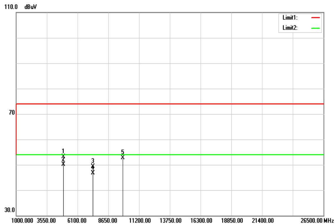
**Operation Mode:** TX / IEEE 802.11b / CH High**Test Date:** June 22, 2016**Temperature:** 27°C**Tested by:** Dennis Li**Humidity:** 53% RH**Polarity:** Ver. / Hor.
