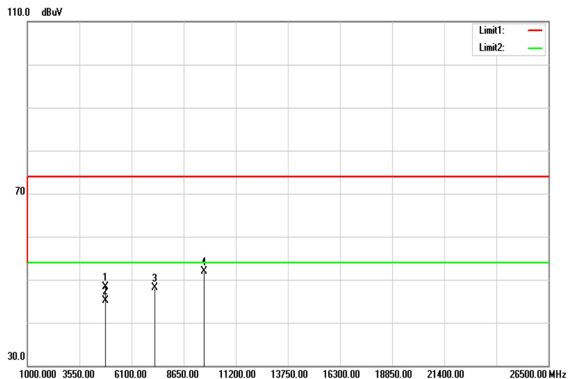
**Operation Mode:** TX / IEEE 802.11g / CH Low**Test Date:** June 22, 2016**Temperature:** 27°C**Tested by:** Dennis Li**Humidity:** 53% RH**Polarity:** Ver. / Hor.
