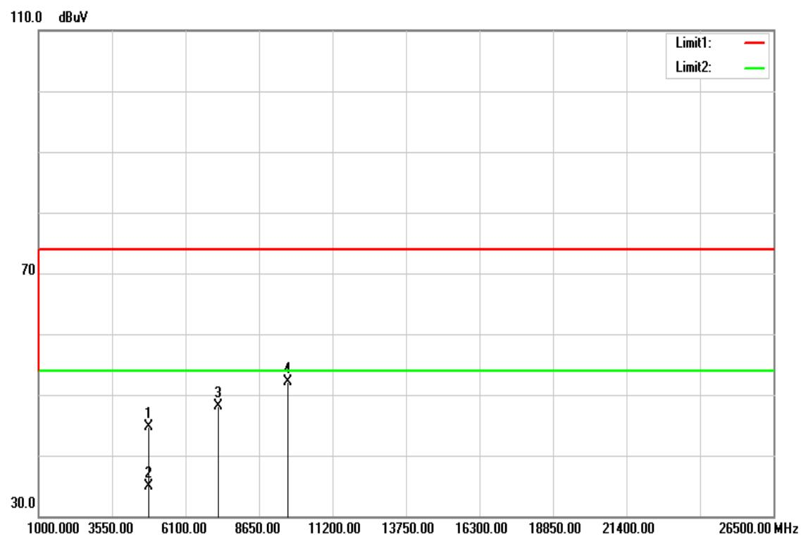
**Operation Mode:** TX / IEEE 802.11n HT 20 MHz mode / CH Low **Test Date:** June 22, 2016
