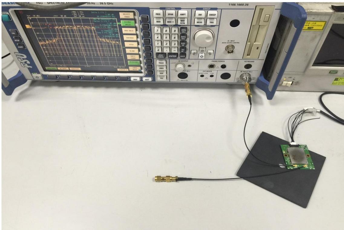
**RADIATED EMISSION SETUP PHOTOS****For PIFA Antenna****Below 1GHz**
