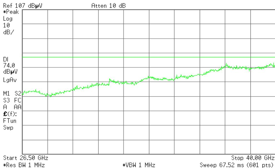
**Operation Mode:** Tx / IEEE 802.11n HT 40 MHz mode / 5510 MHz**Test Date:** January 18, 2016**Temperature:** 27°C**Tested by:** Jason Lu**Humidity:** 53% RH**Polarity:** Ver. / Hor.
