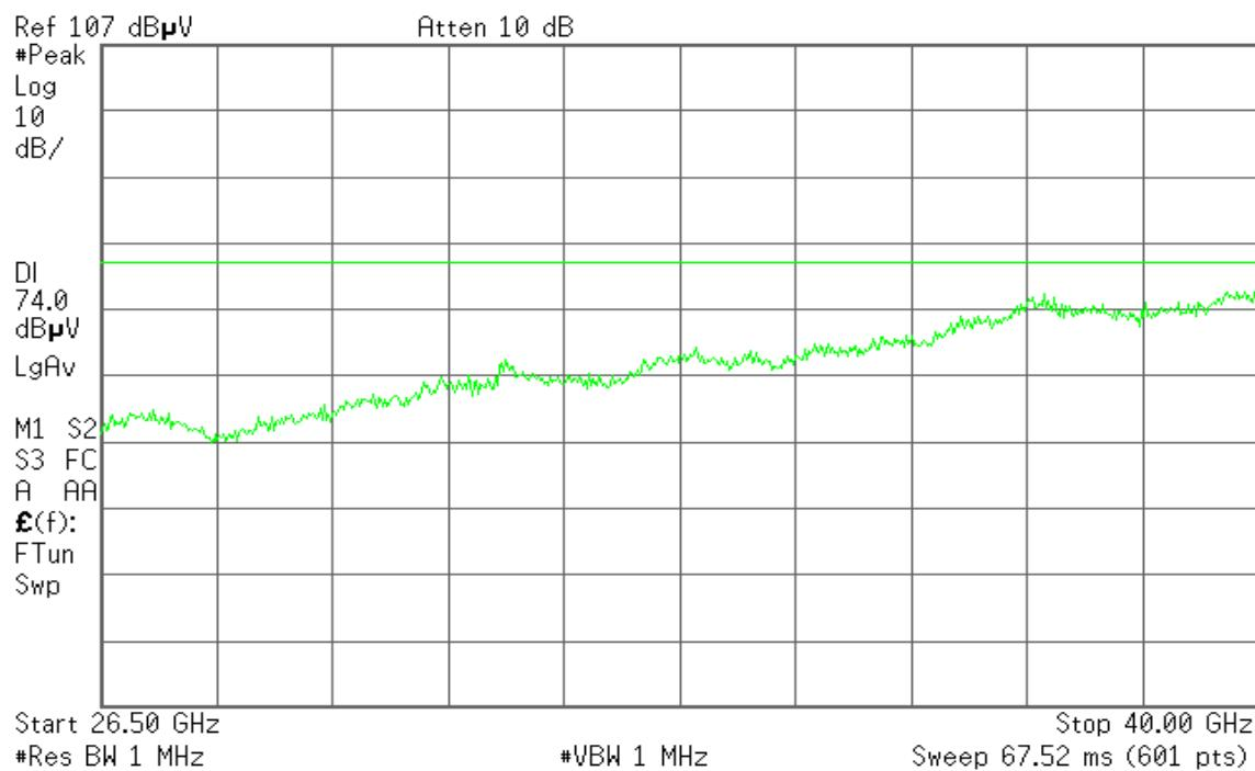
**Operation Mode:** Tx / IEEE 802.11a mode / 5320 MHz    **Test Date:** January 18, 2016
