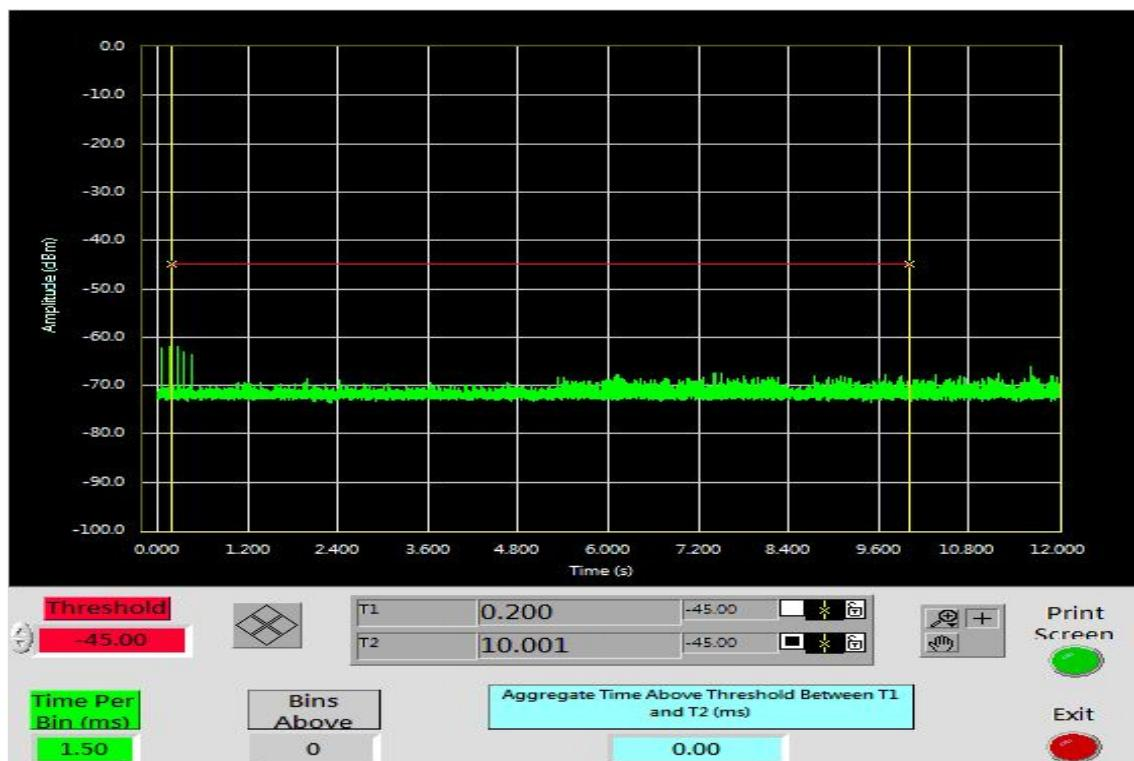
**NON-OCCUPANCY PERIOD****IEEE 802.11n VHT 80 MHz mode****Type 1 Non-Occupancy Period Test Results**
