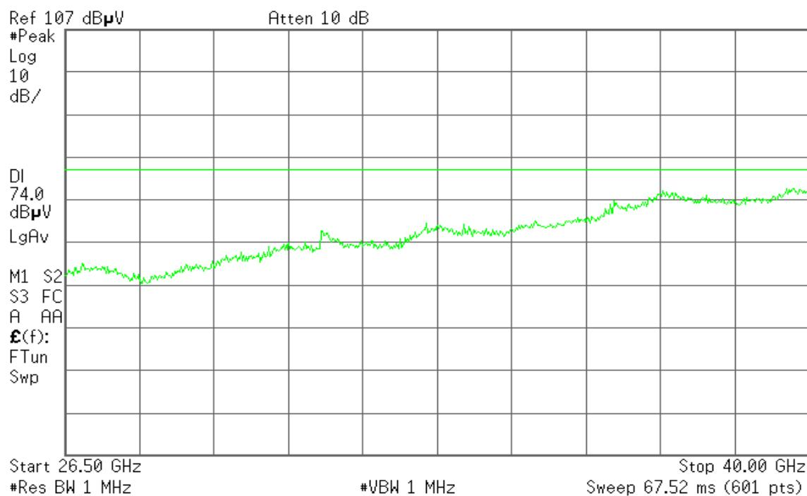
**Operation Mode:** Tx / IEEE 802.11n HT 40 MHz mode / 5510 MHz
