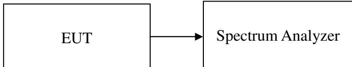
The resolution bandwidth shall be set to as close to 1% of the selected span as is possible without being below 1%. The video bandwidth shall be set to 3 times the resolution bandwidth. Video averaging is not permitted. Where practical, a sampling detector shall be used since a peak or, peak hold.
