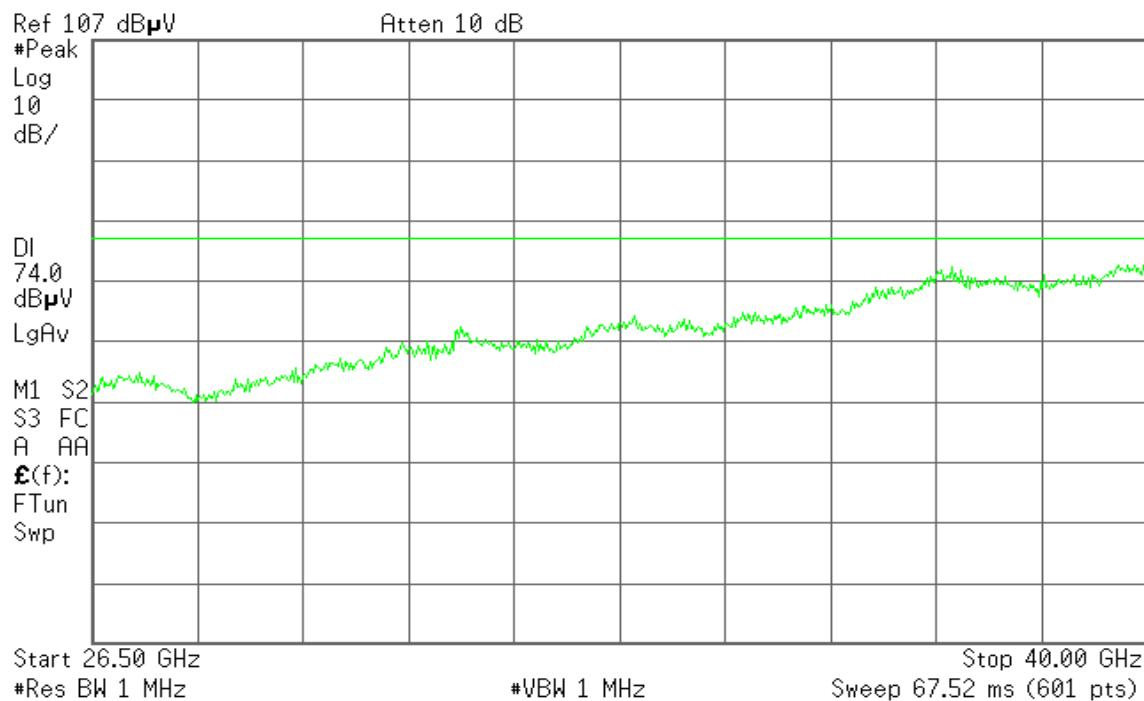
**Operation Mode:** Tx / IEEE 802.11n HT 20 MHz mode / 5240 MHz
