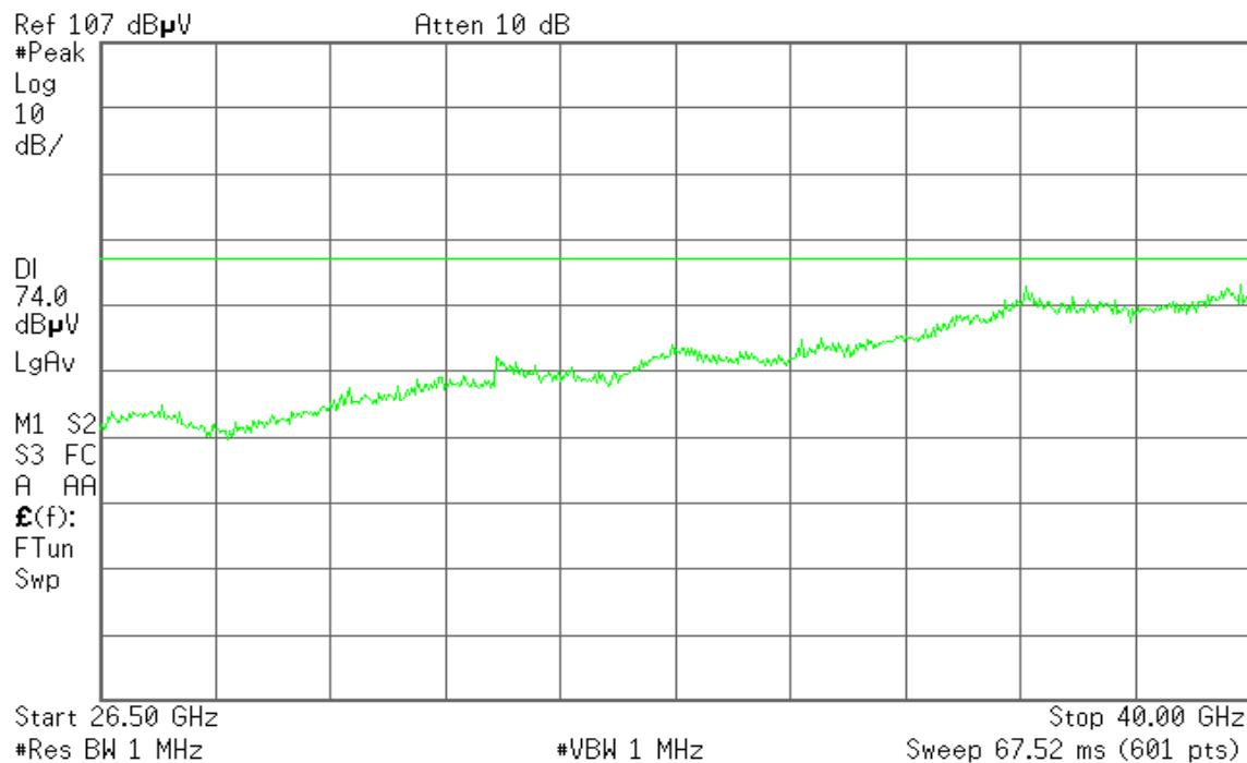
**Operation Mode:** Tx / IEEE 802.11n HT 40 MHz mode / 5270 MHz
