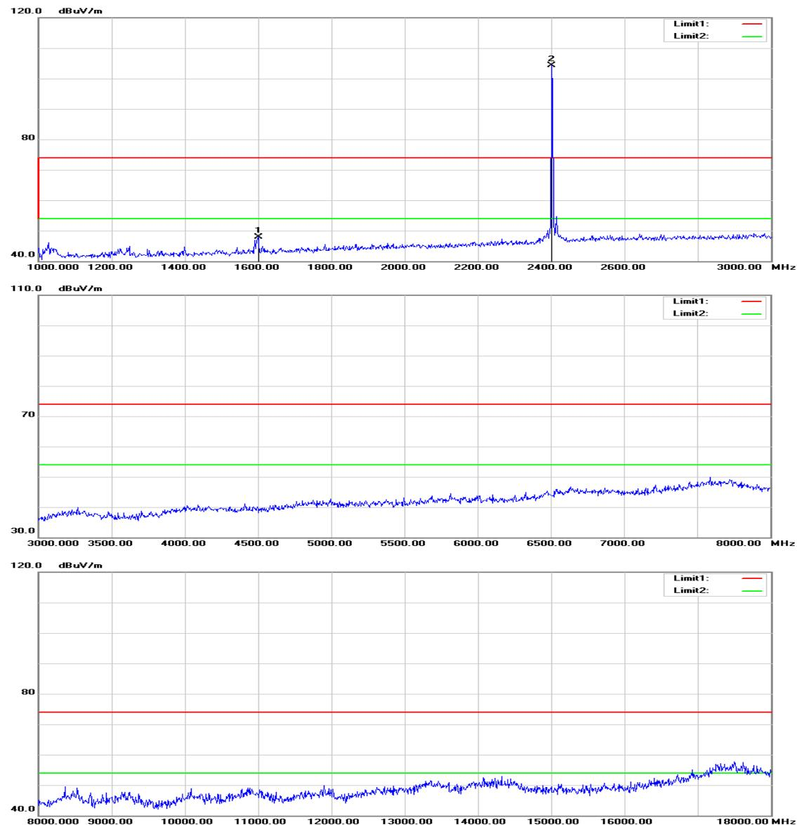
**Above 1 GHz****Operation Mode:** TX / GFSK / DH5 / CH Low**Test Date:** August 25, 2015**Temperature:** 27°C**Tested by:** Jason Lu**Humidity:** 53 % RH**Polarity:** Ver. / Hor.
