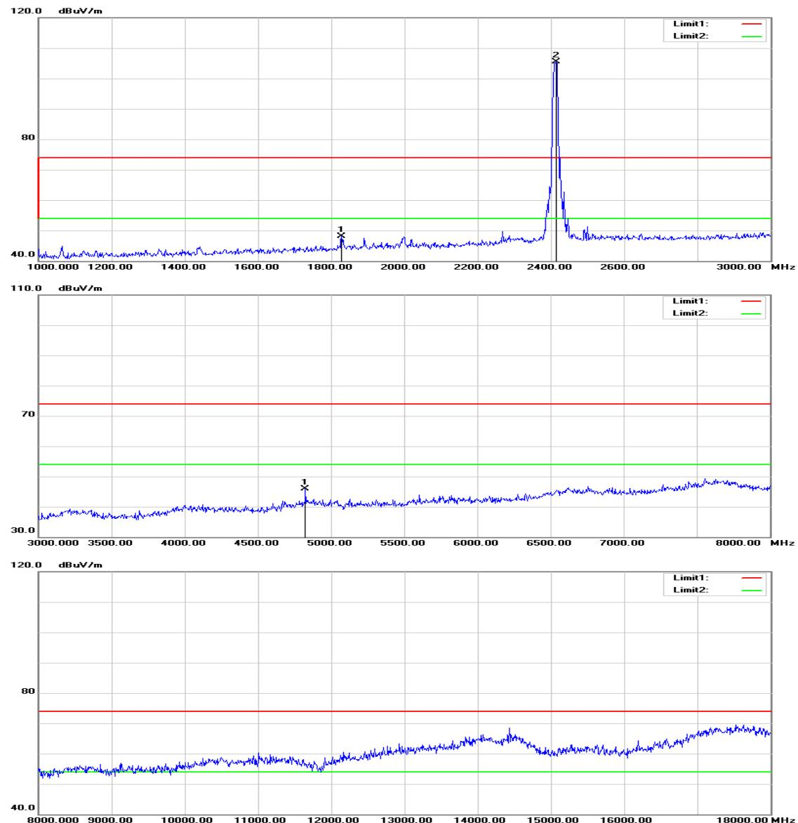
**Above 1 GHz****Operation Mode:** TX / IEEE 802.11b / CH Low**Test Date:** August 25, 2015**Temperature:** 27°C**Tested by:** Jason Lu**Humidity:** 53% RH**Polarity:** Ver. / Hor.
