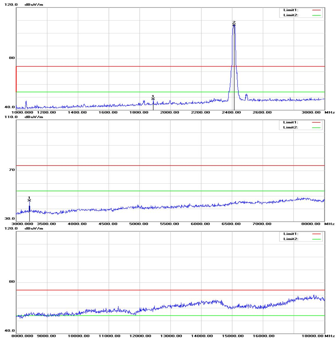
**Operation Mode:** TX / IEEE 802.11g / CH Low**Test Date:** August 25, 2015**Temperature:** 27°C**Tested by:** Jason Lu**Humidity:** 53% RH**Polarity:** Ver. / Hor.
