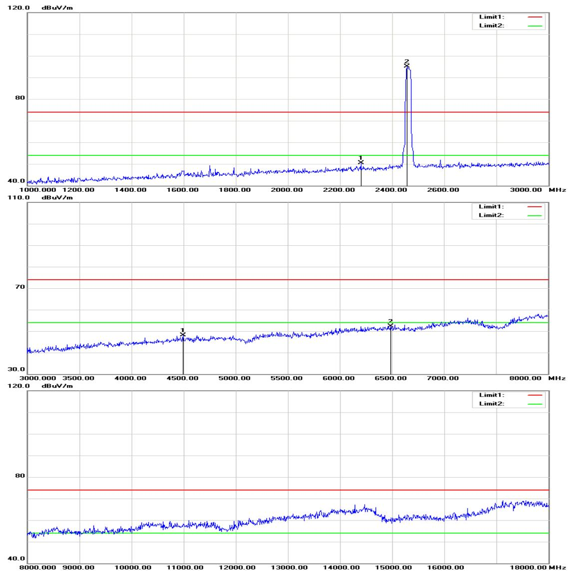
**Operation Mode:** TX / IEEE 802.11g / CH High**Test Date:** August 25, 2015**Temperature:** 27°C**Tested by:** Jason Lu**Humidity:** 53% RH**Polarity:** Ver. / Hor.
