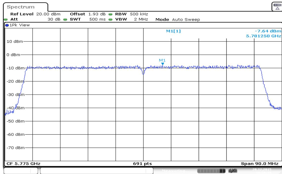
**IEEE 802.11ac VHT 80 MHz mode / 5775MHz / Chain 1****PPSD (CH Mid)**
