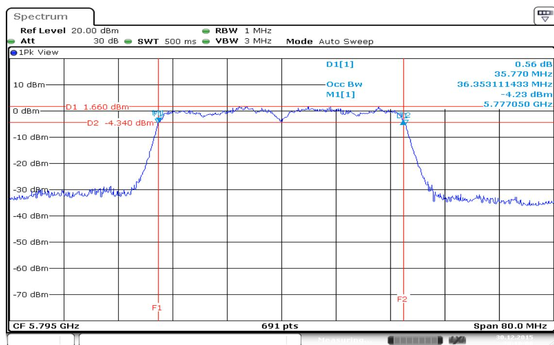
**Test mode: IEEE 802.11ac VHT 80 MHz mode / 5775MHz / Chain 0****99% Bandwidth (CH Mid)**
