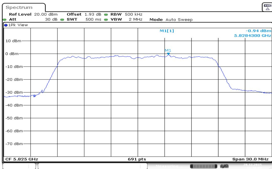
**IEEE 802.11n HT 40 MHz mode / 5755 ~ 5795MHz / Chain 0****PPSD (CH Low)**
