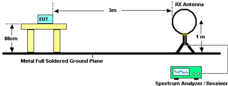
For radiated emissions from 30MHz to 1GHz
