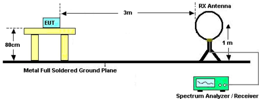
For radiated emissions from 30MHz to 1GHz
