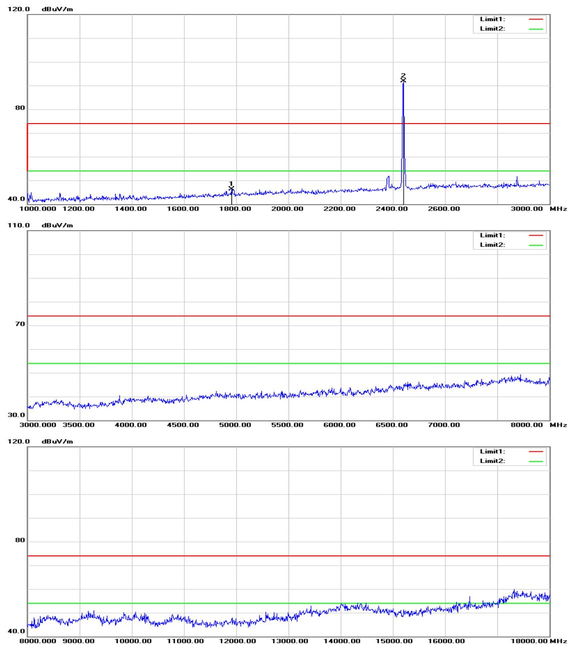
**Operation Mode:** Zigbee / TX / CH Mid**Test Date:** August 18, 2015**Temperature:** 27°C**Tested by:** Jason Lu**Humidity:** 53 % RH**Polarity:** Ver. / Hor.
