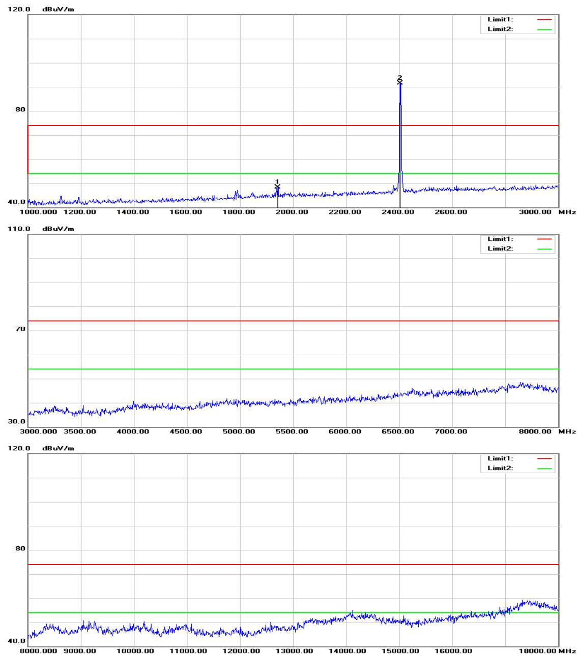
**Operation Mode:** Zigbee / TX / CH Low**Test Date:** August 18, 2015**Temperature:** 27°C**Tested by:** Jason Lu**Humidity:** 53 % RH**Polarity:** Ver. / Hor.
