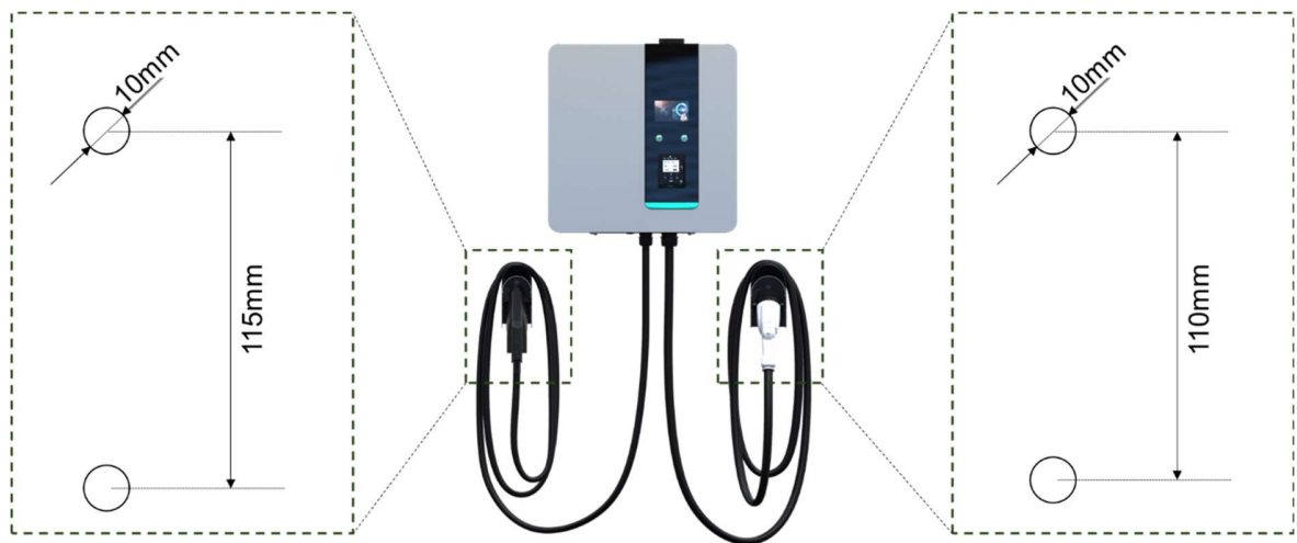
Figure 3-12 Hole Pitch of Holster
