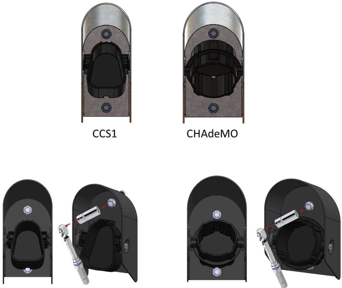
Figure 3-13 Secure the Holster
