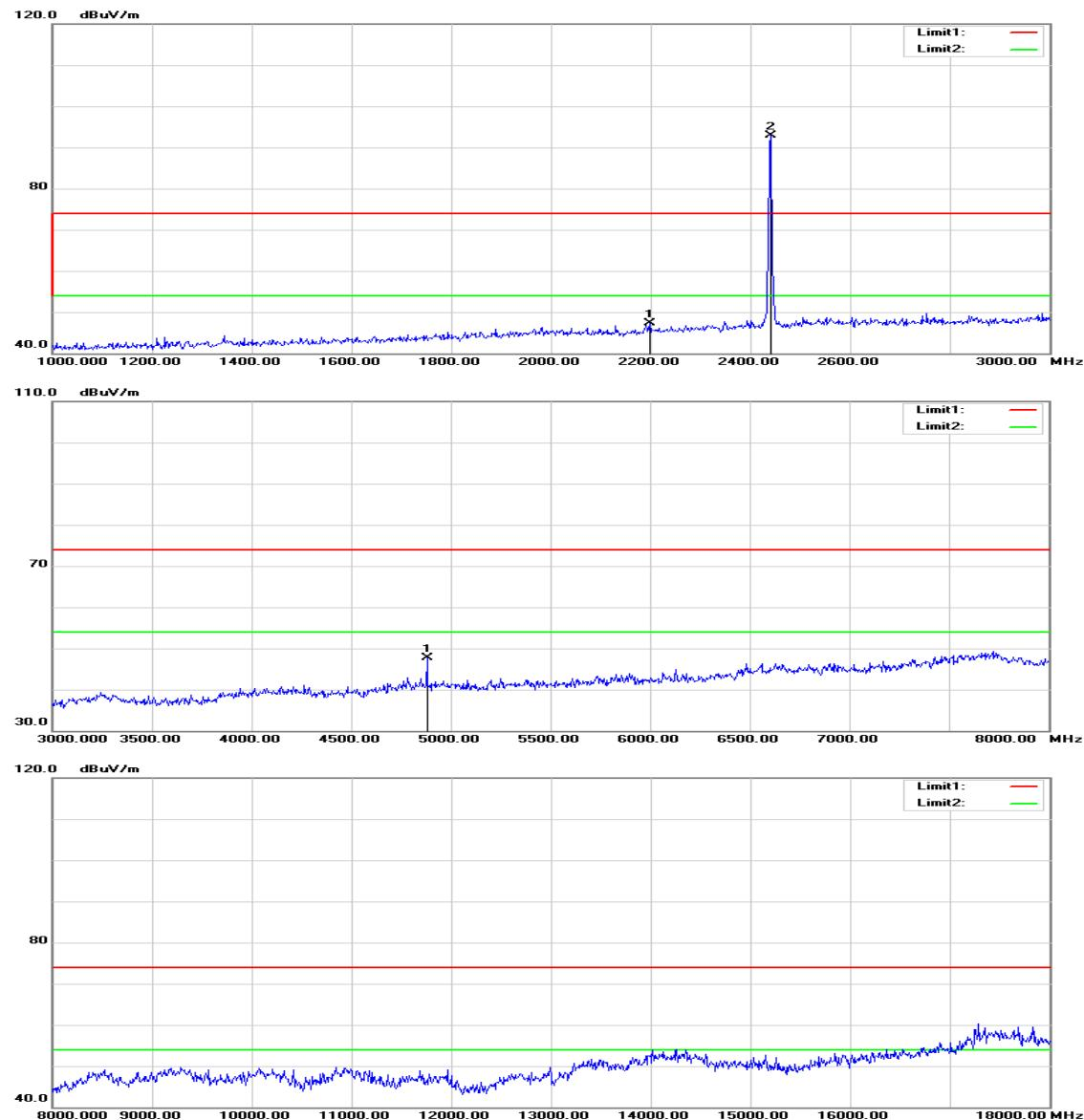
**Operation Mode:** Zigbee / TX / CH Mid**Test Date:** June 23, 2015**Temperature:** 27°C**Tested by:** Jason Lu**Humidity:** 53 % RH**Polarity:** Ver. / Hor.
