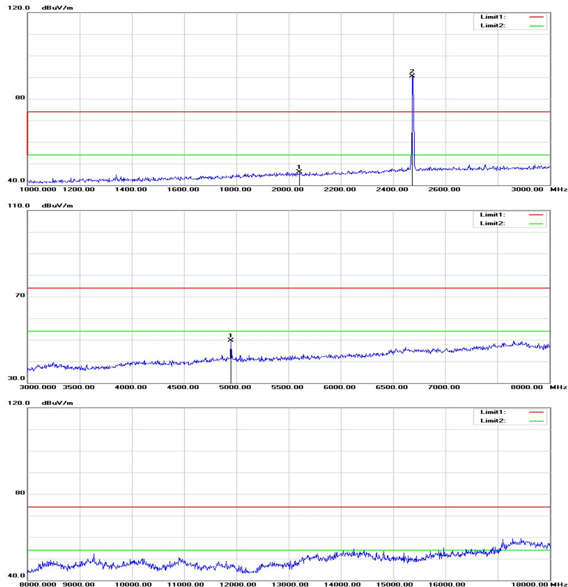
**Operation Mode:** Zigbee / TX / CH High**Test Date:** June 23, 2015**Temperature:** 27°C**Tested by:** Jason Lu**Humidity:** 53 % RH**Polarity:** Ver. / Hor.
