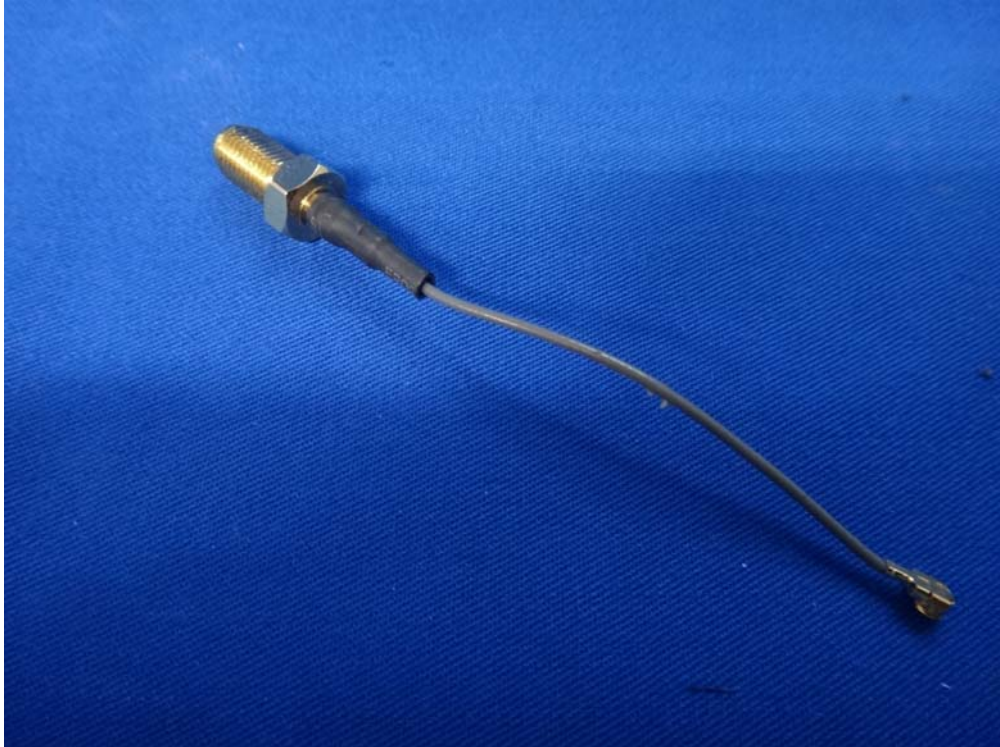
(13) EUT Photo (Antenna: RFDPA520900SMAB601)
