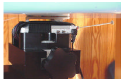
Body SAR Test Setup with 1.4cm Belt-Holster
