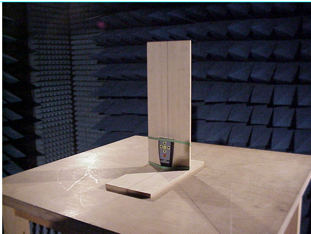
Particular of EUT test set-up arrangement during the test
