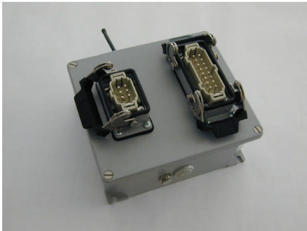
The receiver unit Series **FreeHand** may be **12 VDC** or **24 VDC** (this latter on request) power supplied, through a connection to the battery of the means where it's installed.
