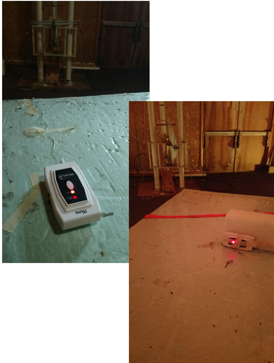
Figure 4: Radiated Emissions Test Setup Photograph(s).
