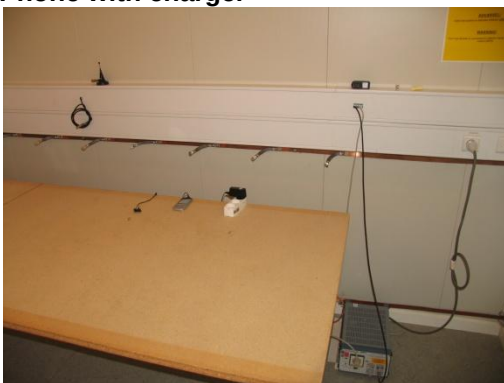
Picture(s) 3. FCC Part 15C AC powerline conducted emissions Phone with charger
