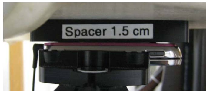
Photo of the device positioned for Body SAR measurement. The spacer was removed for the tests.
