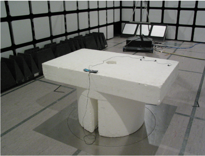
Picture 3 Radiated emission measurement GSM RX + FM radio on
