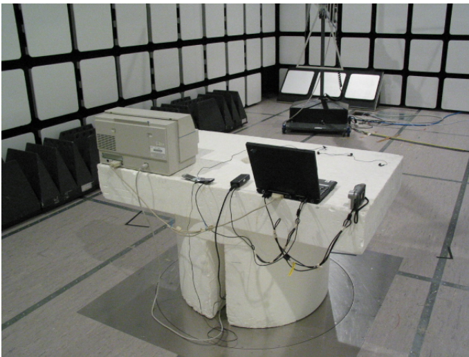
Picture 2 Radiated emission measurement GSM RX + Computer peripherals
