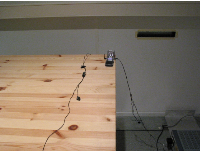
Picture 4 AC powerline conducted emission measurement Bluetooth TX
