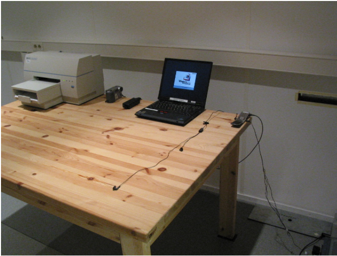
Picture 5 AC powerline conducted emission measurement GSM RX + Computer peripherals
