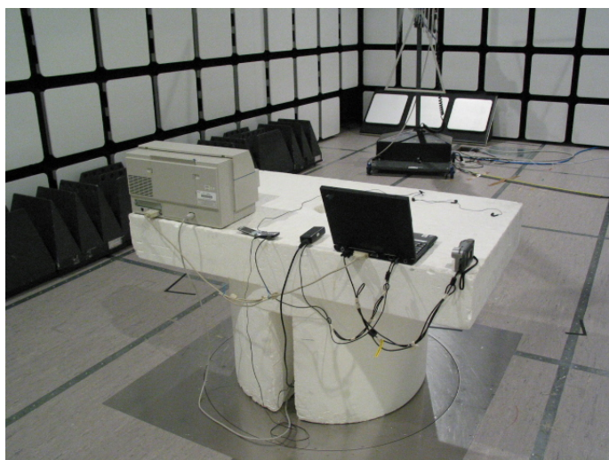
Picture 2 Radiated emission measurement GSM RX + Computer peripherals
