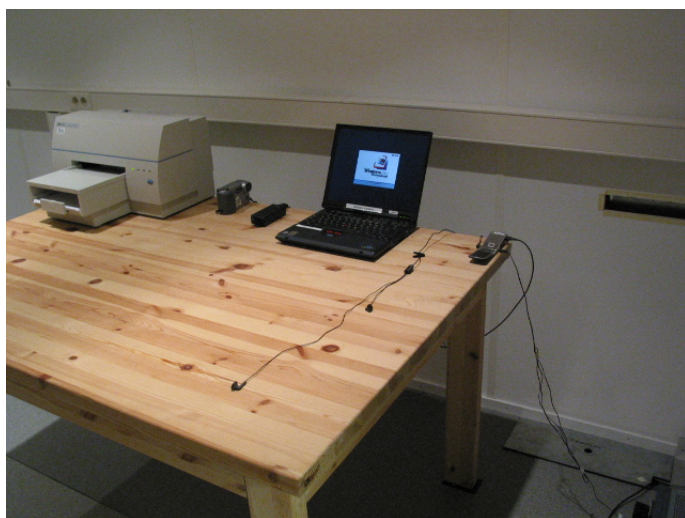
Picture 5 AC powerline conducted emission measurement GSM RX + Computer peripherals
