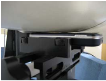
Photo of the device closed in "cheek" position
