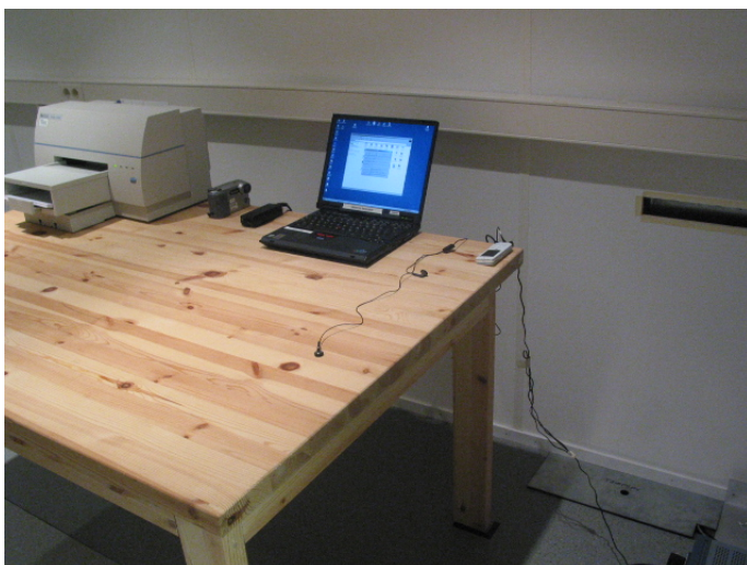
Picture 4 AC powerline conducted emission measurement GSM RX / Bluetooth TX + Computer peripherals
