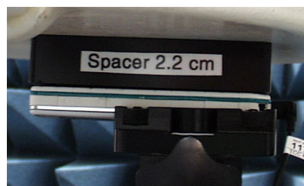
Photo of the device positioned for Body SAR measurement. The spacer was removed for the tests.
