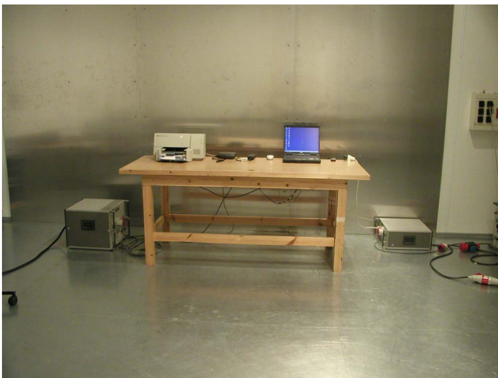
Photograph 1. AC power line conducted emissions test setup
