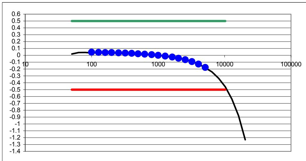
Result: The raw frequency response of the uncompensated probe system in the range 100 Hz to 10 kHz is < 0.5 dB. The correlation with the measurements above is excellent.
