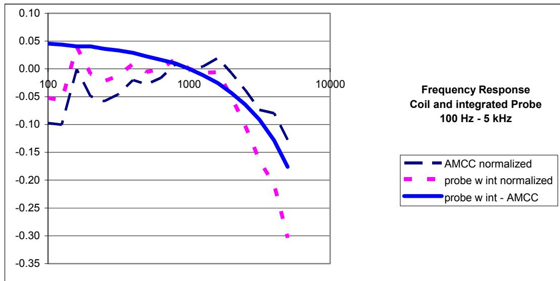
Remarks: Normalizations are to 1 kHz. An AMCC voltage of -20 dB V is equivalent to 1 A/m. Calibration level is -8.1 dB A/m = 0.39 A/m.
