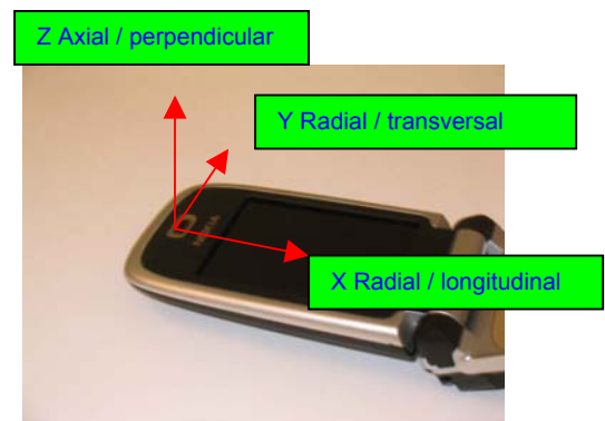
Photo of the device positioned under Test Arch and coordinate system
