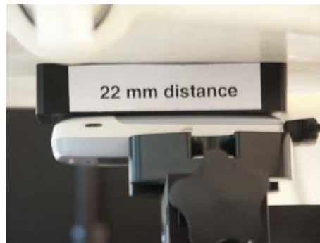
Photo of the device positioned for Body SAR measurement.
