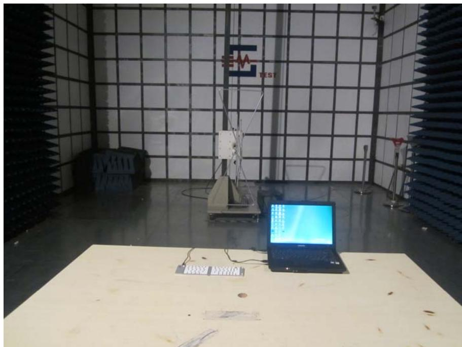
**Radiation Emission Test Setup (9kHz to 30MHz)**
