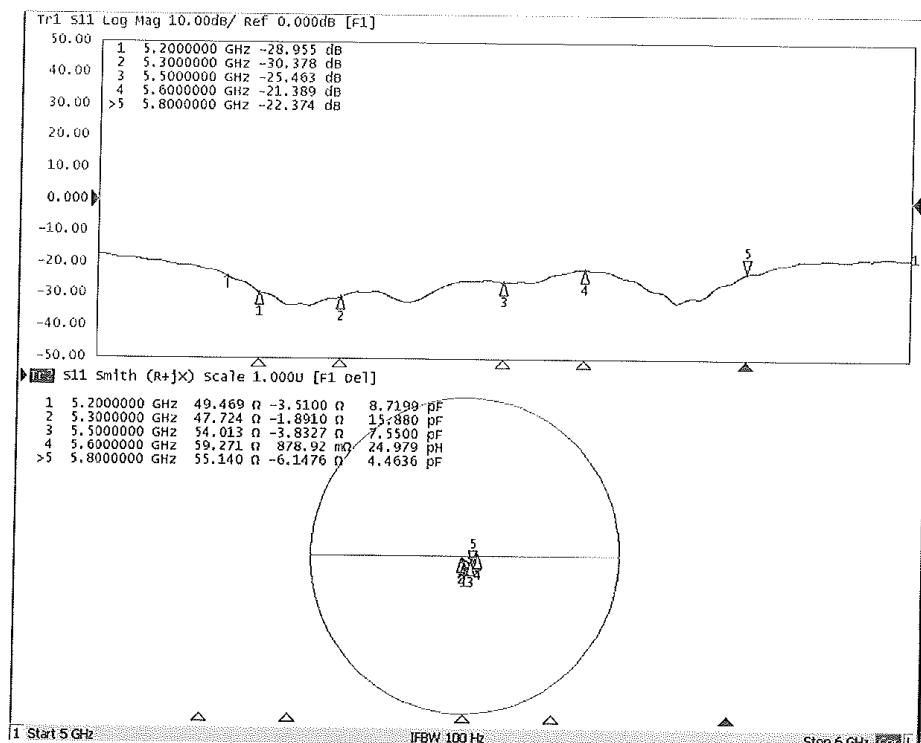
**D5GHzV2, Serial No.1095 Extended Dipole Calibrations**
