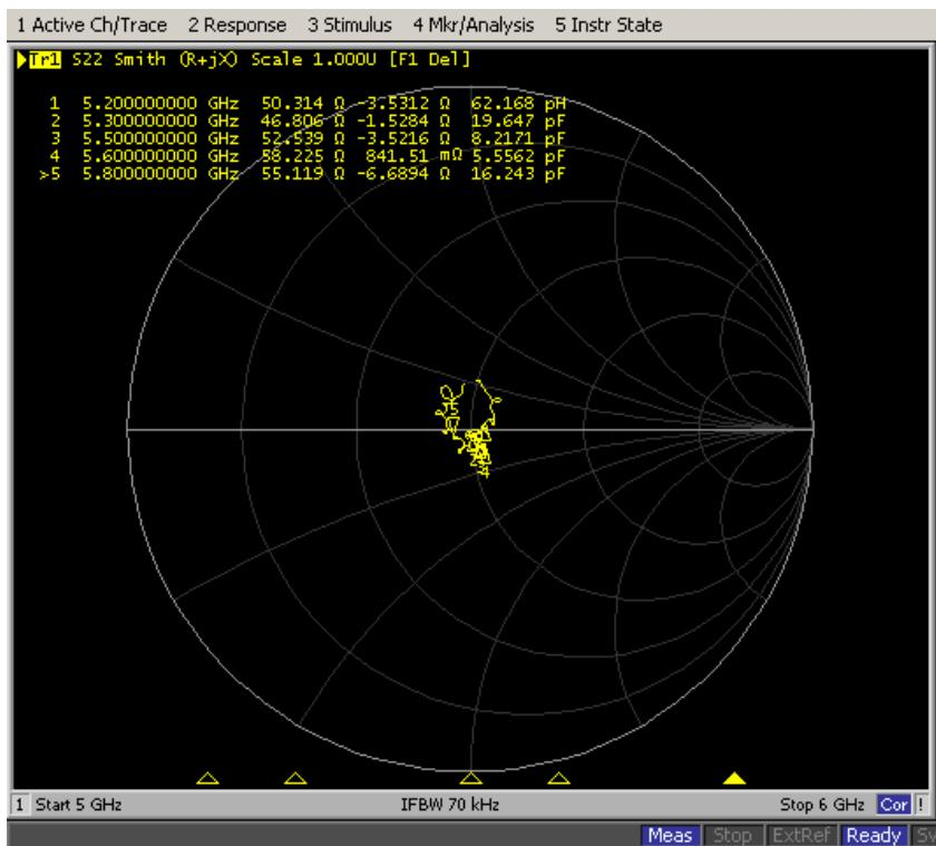
**D5GHzV2,Serial No.1095 Extended Dipole Calibrations**
