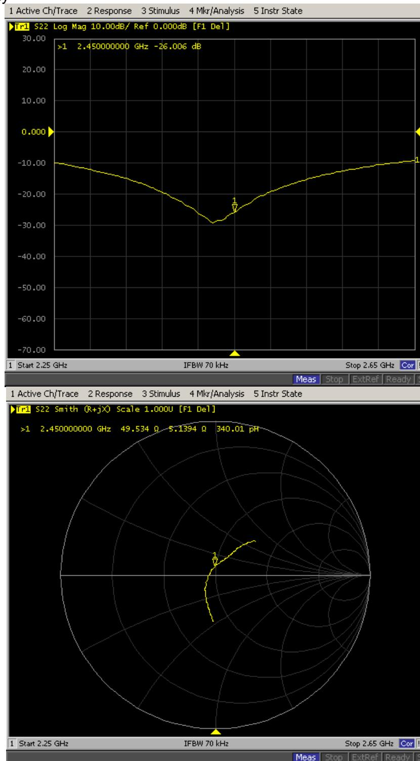
**D2450V2, Serial No.817 Extended Dipole Calibrations**
