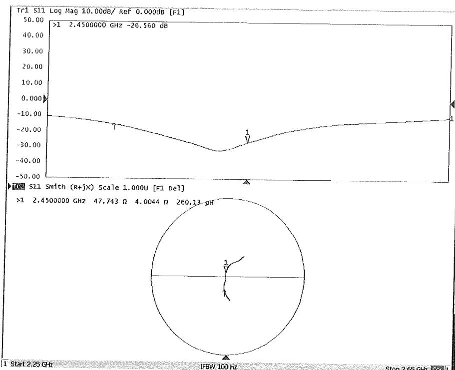
**D2450V2, Serial No.817 Extended Dipole Calibrations**
