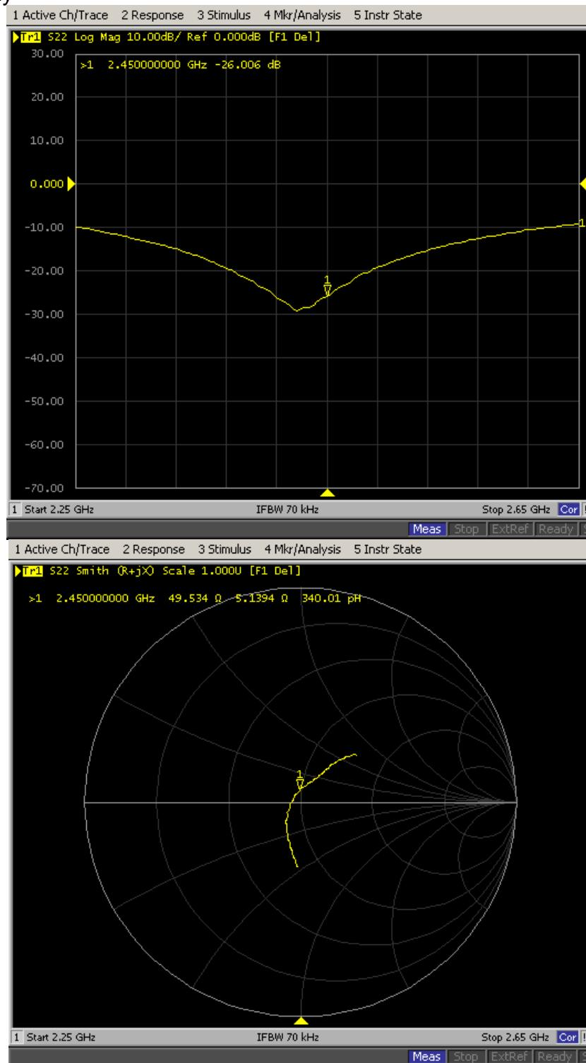
**D2450V2, Serial No.817 Extended Dipole Calibrations**
