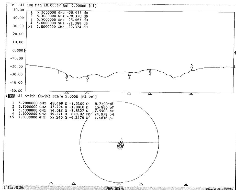
**D5GHzV2, Serial No.1095 Extended Dipole Calibrations**
