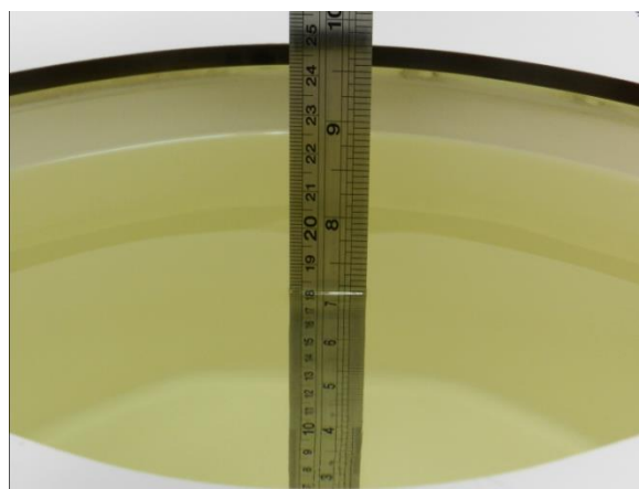
Fig 10.2 Photo of Liquid Height for Body SAR
