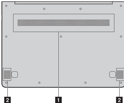
**1 Ventilation slots** Dissipate internal heat.
