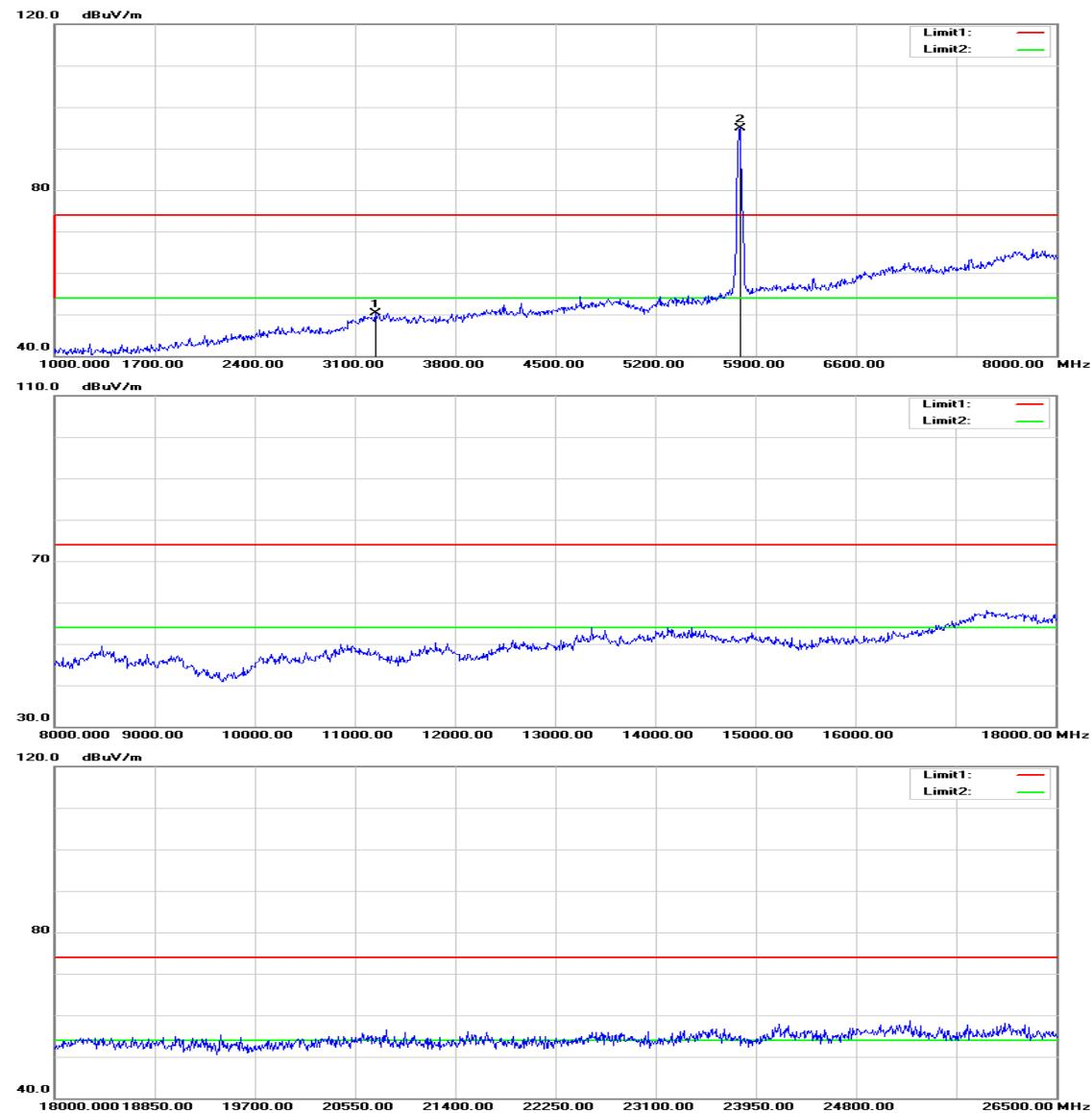
**Operation Mode:** TX / IEEE 802.11a mode / CH Mid**Test Date:** July 29, 2015**Temperature:** 27°C**Tested by:** Owen Wu**Humidity:** 53% RH**Polarity:** Ver. / Hor.
