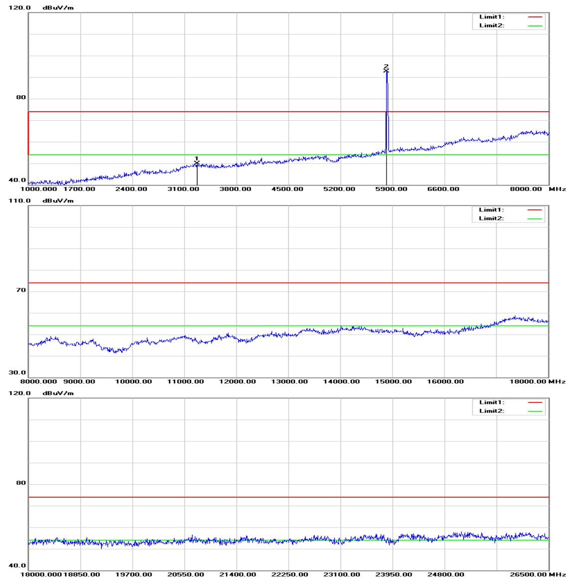
**Operation Mode:** TX / IEEE 802.11a mode / CH High**Test Date:** July 29, 2015**Temperature:** 27°C**Tested by:** Owen Wu**Humidity:** 53% RH**Polarity:** Ver. / Hor.
