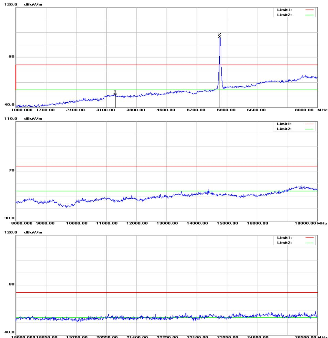
**Operation Mode:** TX / IEEE 802.11a mode / CH Low**Test Date:** July 29, 2015**Temperature:** 27°C**Tested by:** Owen Wu**Humidity:** 53% RH**Polarity:** Ver. / Hor.
